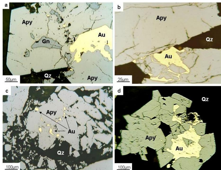
**Figure 3.** Typical mineral intergrowths of native gold in ores of gold–arsenic-sulfide GIT deposits: (a) intergrowth with arsenopyrite (Nataalka); (b) development of native gold along cracks in arsenopyrite (Karalveem); (c) small inclusions of native gold in a single crystal of arsenopyrite (Degdekan); (d) overlay of native gold on an intergrowth of arsenopyrite crystals (Maldyak).
