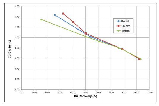
**Figure 6.** Cumulative grade-recovery curves for the overall sample as well as the +40 mm and -40 mm size fractions.
