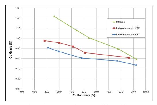
Figure 8. Cumulative grade-recovery curves for the intrinsic and laboratory (ideal) sensor tests.
