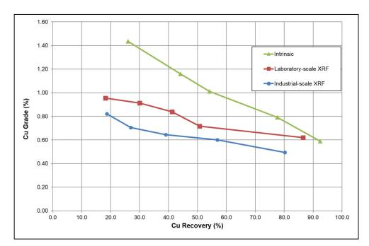
**Figure 9.** Cumulative grade-recovery and mass rejection curves for the intrinsic, ideal and industrial sensor tests.
