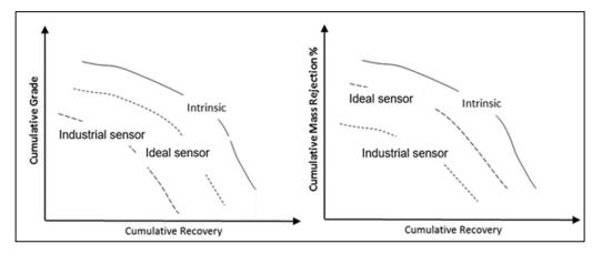
**Figure 3.** Examples of cumulative grade, recovery and mass rejection curves comparing the intrinsic, ideal sensor and industrial sensor sortability tests.
