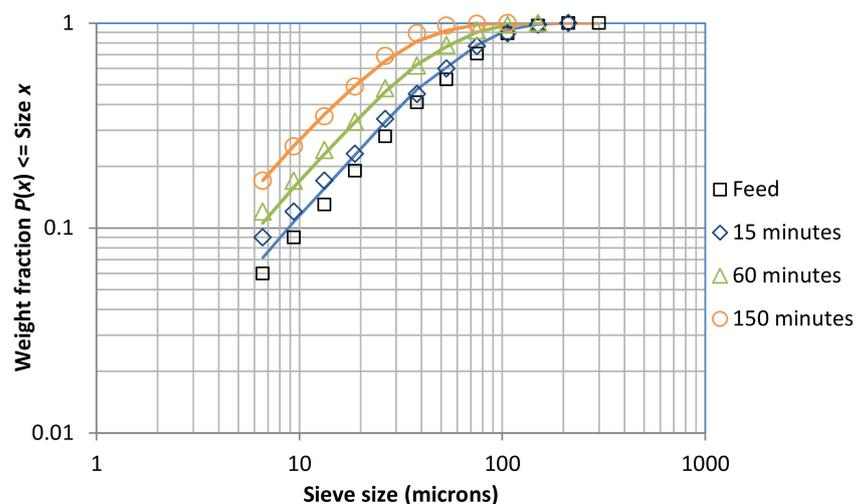
**Figure 6.** Product size distributions at grinding times 0 (feed), 15, 60 and 150 min; symbols are experimental data, lines the model values ( $a = 7.6 \times 10^{-5} \text{ min}^{-1}$ ,  $\alpha = 1.27$ , Run 1).
