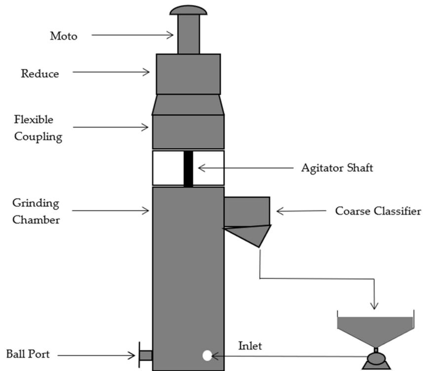
Figure 3. Illustration of the Kubota Tower mill rigged to operate as a batch mill.
