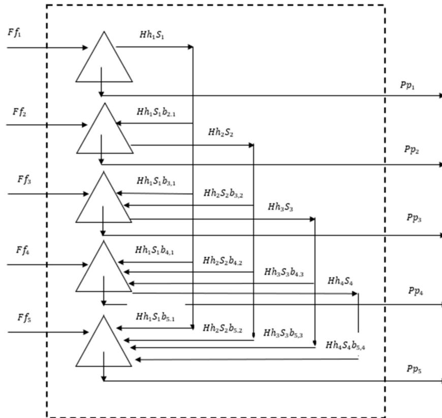
**Figure 1.** The classic size-mass balance model. The model depicts a perfectly mixed mill region, represented by the dotted line, with each size range within the region represented as a triangle. The arrows represent the contributions from a feed stream and to a product stream and the internal flows from and to each size class.
