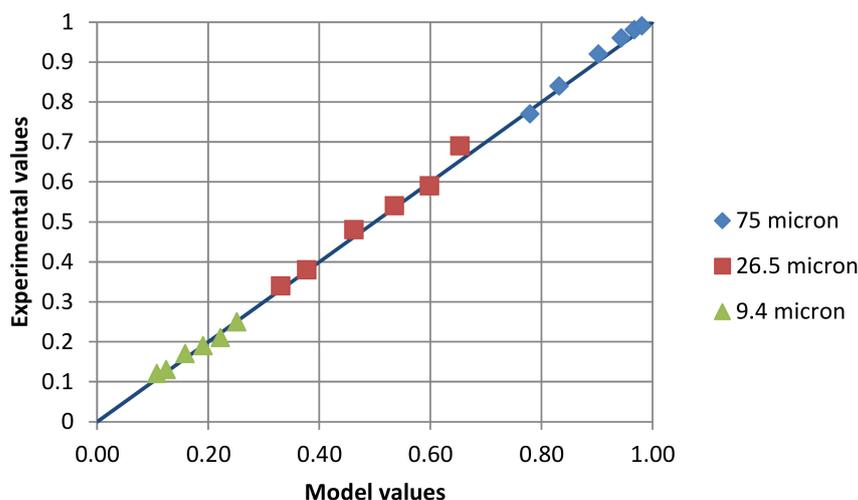
**Figure 7.** Experimental values of % < size versus predicted model values, for sizes  $x_i = 75, 26.5$  and  $9.4$  microns, for the six grinding times ( $a = 7.6 \times 10^{-5} \text{ min}^{-1}$ ,  $\alpha = 1.27$ , Run 1).
