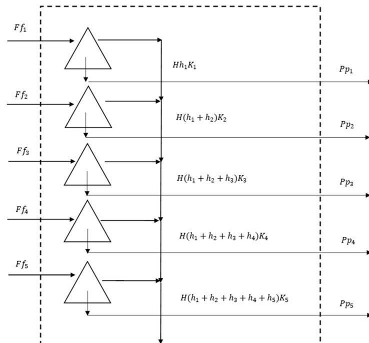
**Figure 2.** The simple model. The model depicts a perfectly mixed mill region, represented by the dotted line, with each size range within the region represented as a triangle. The arrows represent the contributions from a feed stream and to a product stream.
