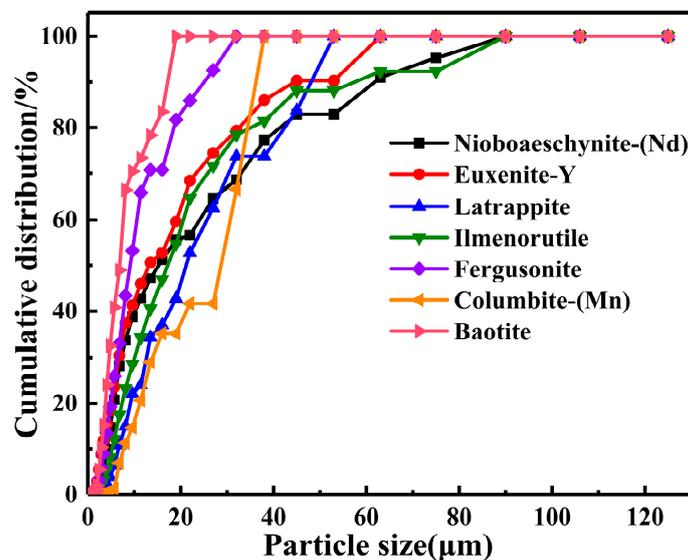
Figure 6. Cumulative particle size distributions of niobium-bearing minerals.
