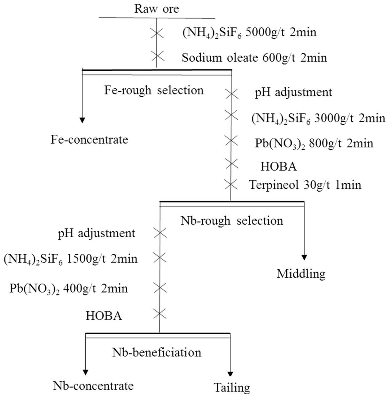
Figure 1. The flowsheet of the flotation of niobium-containing minerals.
