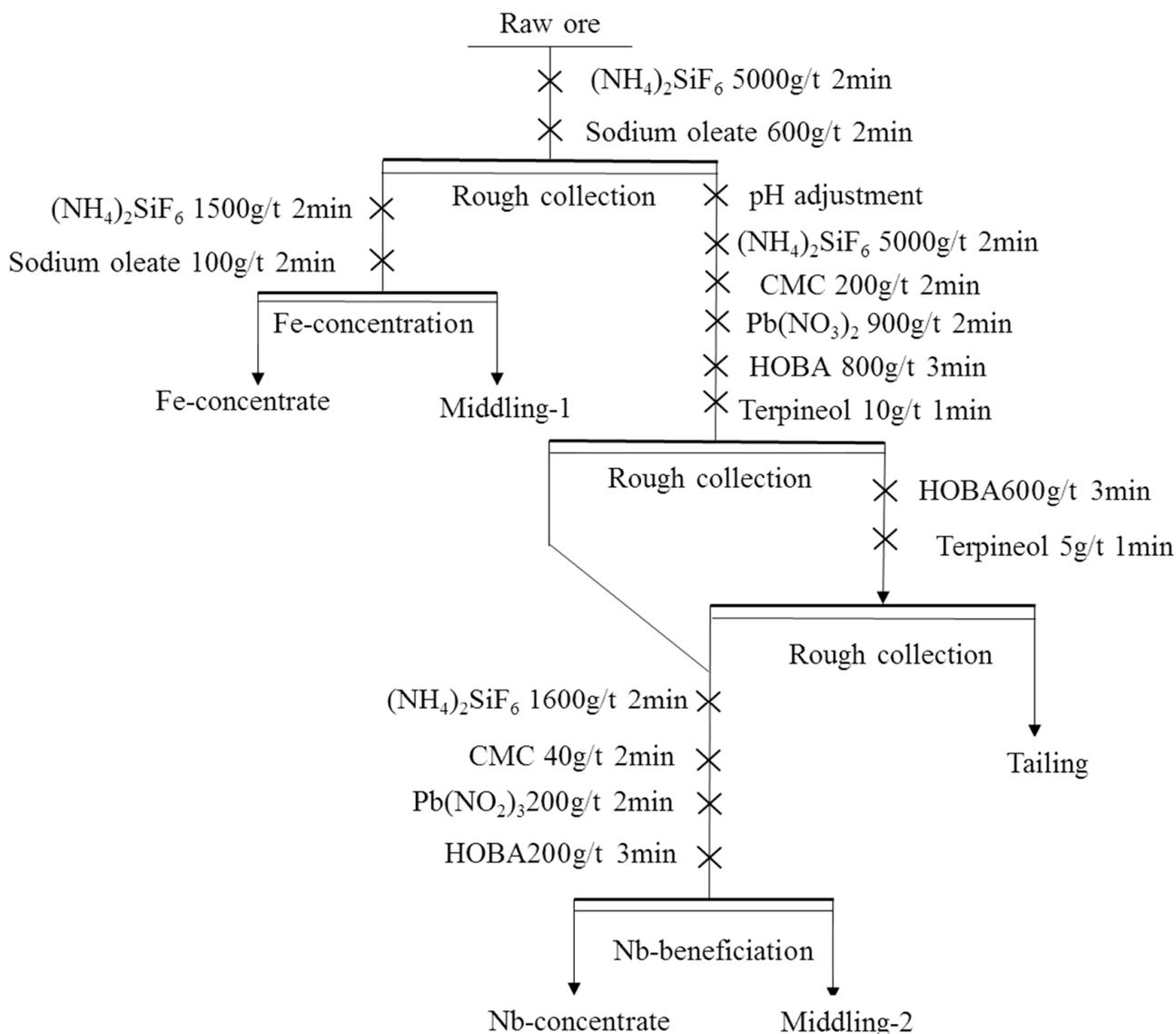
Figure 2. The flowsheet of the flotation optimization experiments.
