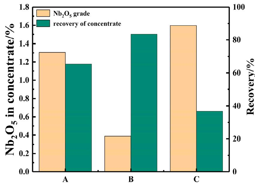
**Figure 10.** Comparison of flotation effects of three flotation collectors. (A: HOBA; B: octyl isohydroxamic acid; C: salicylic hydroxamic acid).
