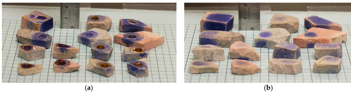
**Figure 8.** (a) Top surface of thick slabs with ink dimples; (b) Bottom surface of slabs showing ink breakthrough. Exposure times from six hours to three days. Top row of samples, left to right: pink, gray pink; Second row: gray, gray pink; Third row: gray, pink, gray, gray; Bottom row: gray, pink, gray, gray.
