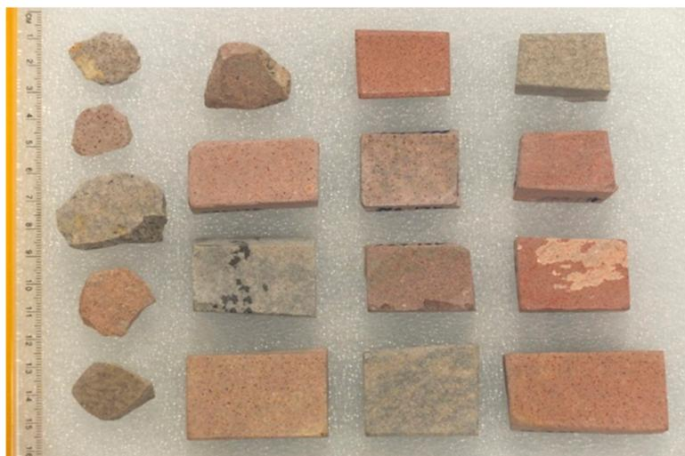
**Figure 2.** Polished blocks and specimens of pink (including red and purple hues) and gray varieties of Round Top Mountain rhyolite. Note sub-mm size of the mineral grains. Scale = 16 cm.
