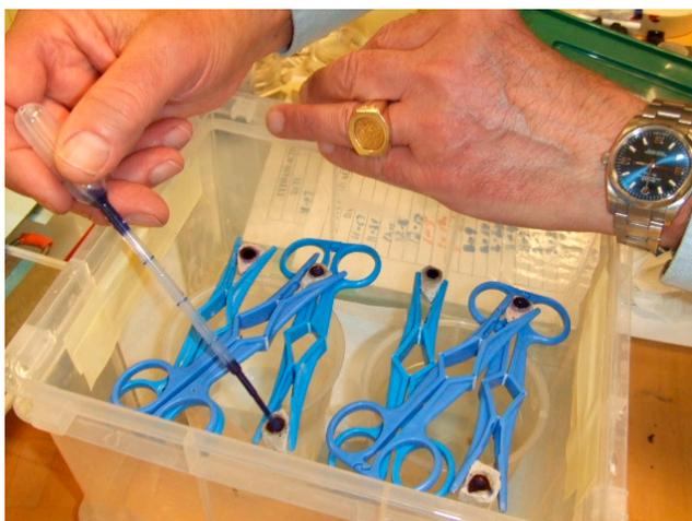
**Figure 4.** Drops of fountain pen ink being applied to thick slabs of rhyolite in the open humidifying box. Beakers of water to maintain humidity visible at the bottom of box.
