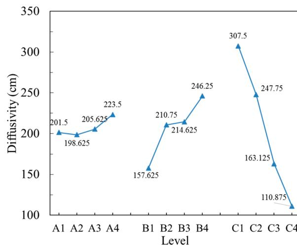
**Figure 7.** The average diffusivity of the slurry at each level.
