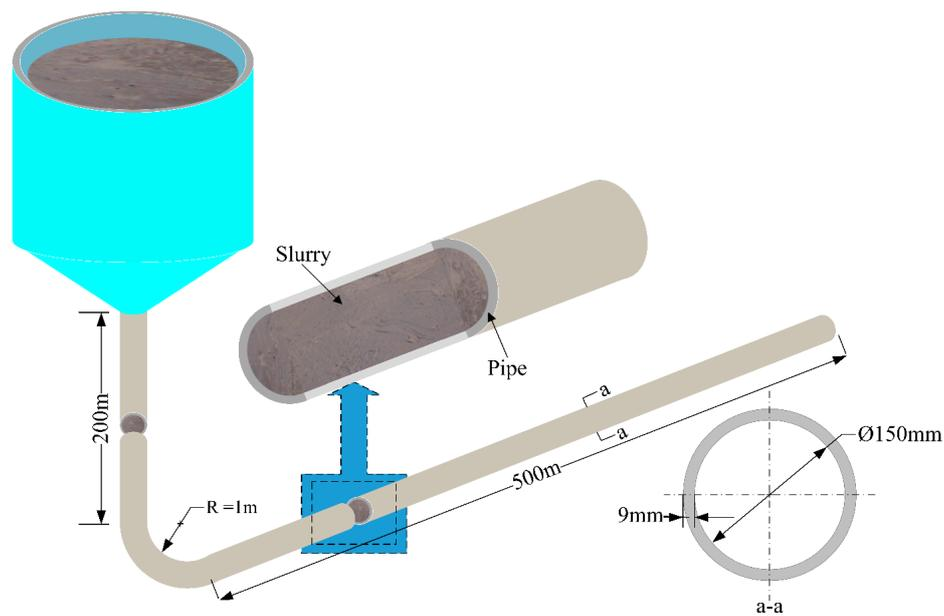
Figure 4. The diagram of the pipeline transport system.
