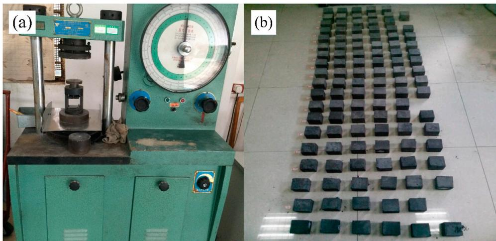
**Figure 2.** Pressure testing machine and test block: (a) pressure testing machine and (b) test block.
