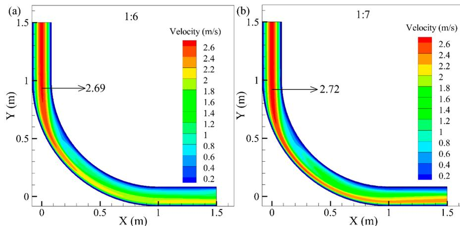
**Figure 8.** Velocity contours at the elbow for different leaching residue:classified tailings mass ratios: (a) 1:6 and (b) 1:7.
