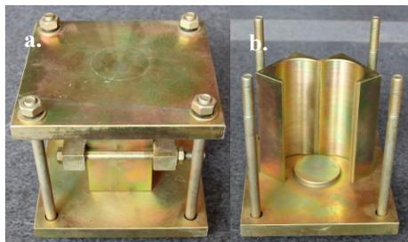
**Figure 1.** Device for cemented paste backfill (CPB) specimen production. Closed state (a); Open state (b).
