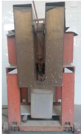
**Figure 1.** The device used for kerosene magnetizing treatment.
