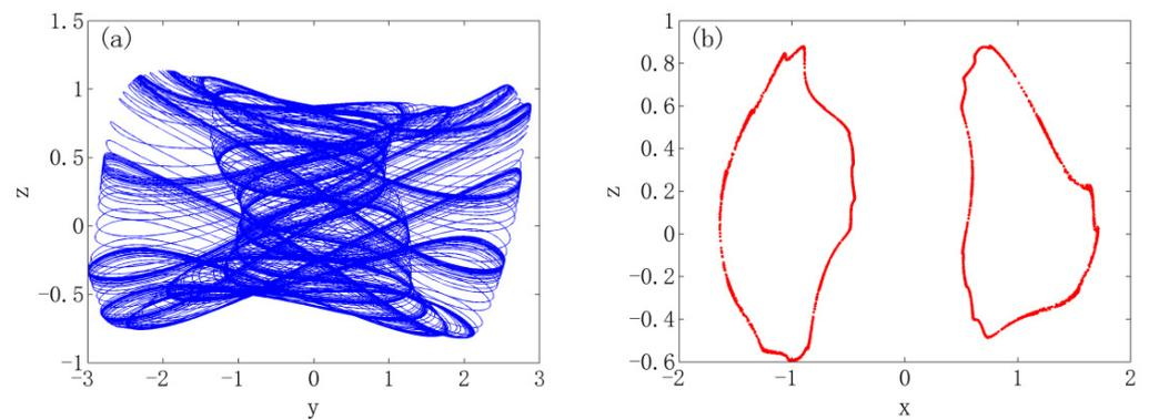
**Figure 8.** Hidden quasi-periodic attractor of system (4) when  $\beta = 0.58$ . (a) Phase trajectory diagram in  $yz$  plane; (b) Poincaré map in  $xz$  plane.
