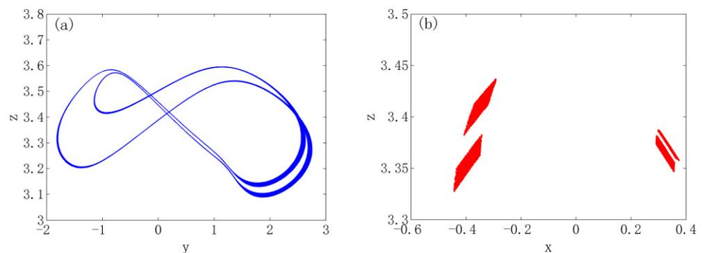
**Figure 1.** Hidden chaotic attractor of system (4) when  $\alpha = 0.28$ . (a) Phase trajectory diagram in  $yz$  plane; (b) Poincare map in  $xz$  plane.
