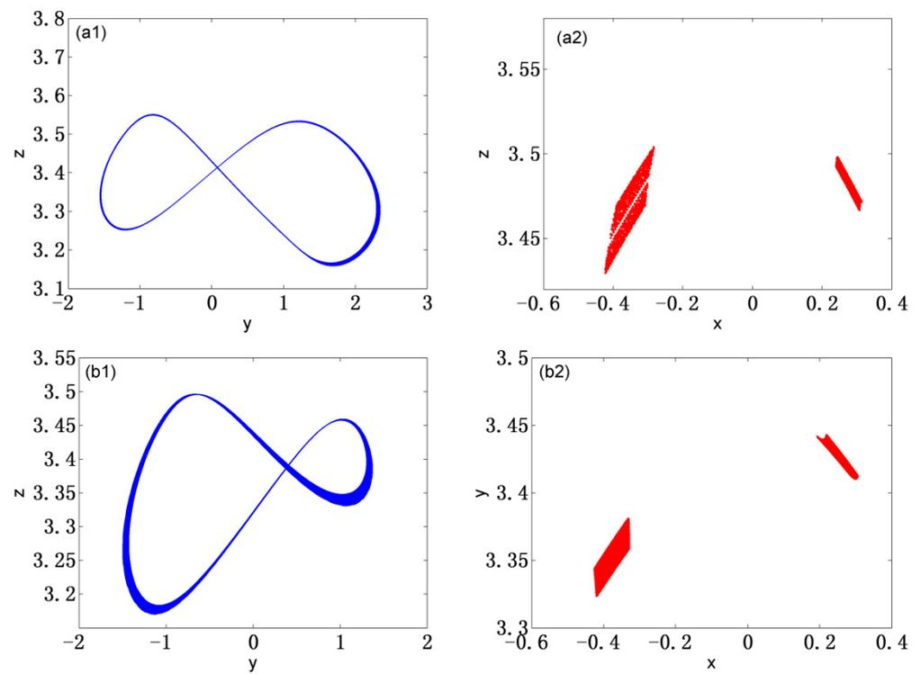
**Figure 11.** Coexistence of hidden chaotic attractors with symmetrical structure for different initial values. (a1,a2) are phase trajectory and Poincare maps with initial value (0, 2, 0, 0), respectively. (b1,b2) are phase trajectory and Poincare maps with initial value (1, -2, 0, 1), respectively.
