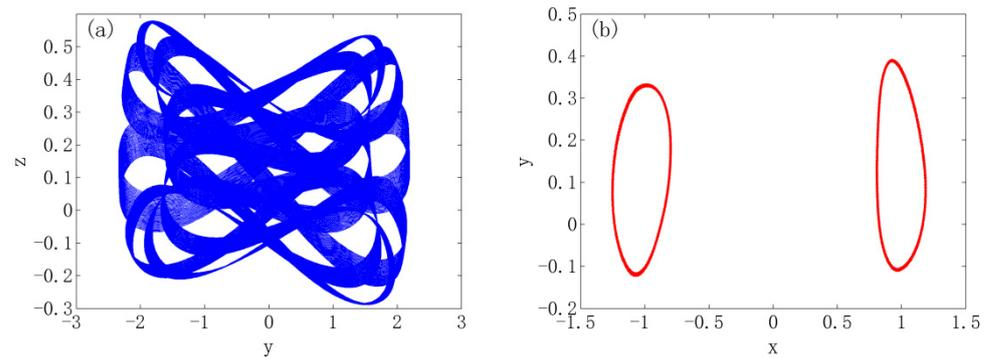
**Figure 3.** Hidden quasi-periodic attractor of system (4) when  $\alpha = 0.95$ . (a) Phase trajectory diagram in  $yz$  plane; (b) Poincare map in  $xz$  plane.
