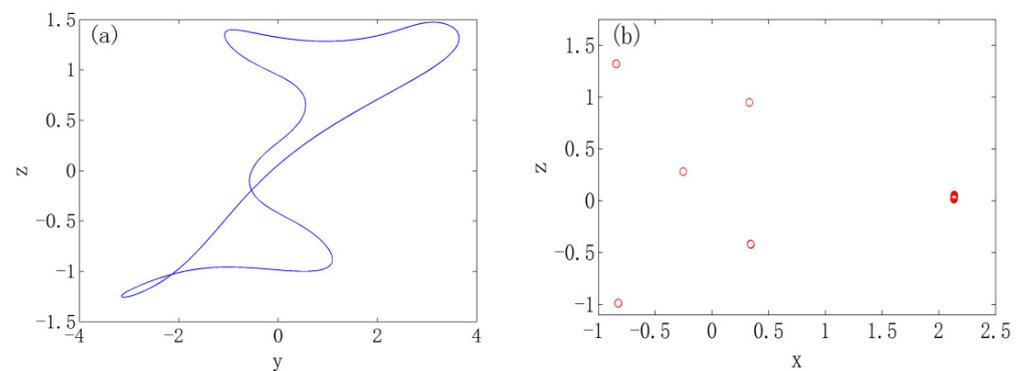
**Figure 7.** Hidden periodic attractor of system (4) when  $\beta = 0.4$ . (a) Phase trajectory diagram in  $yz$  plane; (b) Poincaré map in  $xz$  plane.
