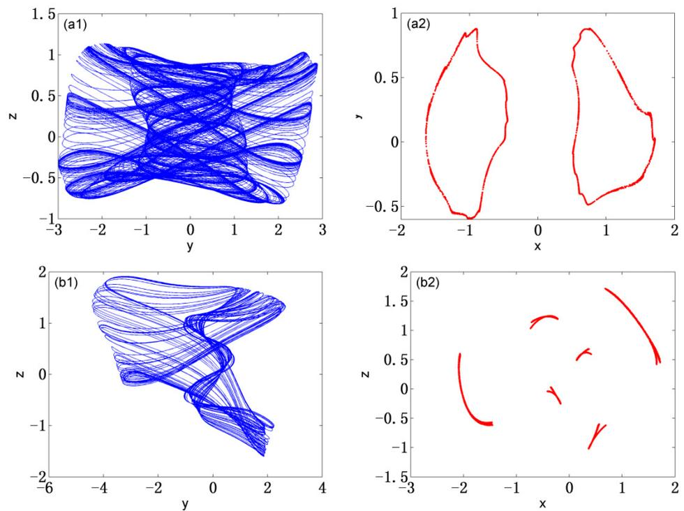
**Figure 12.** Coexistence of hidden quasi-periodic and chaotic attractor for different initial values. (a1,a2) are phase trajectory and Poincare maps with initial value (0, 2, 0, 0), respectively. (b1,b2) are phase trajectory and Poincare maps with initial value (1, -2, 0, 0), respectively.
