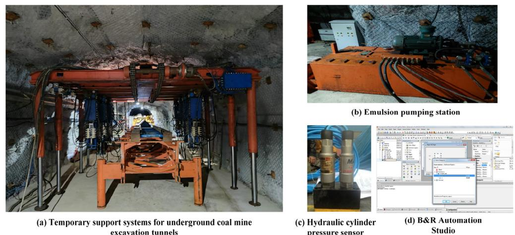
**Figure 18.** Schematic diagram of the composition of the experimental system.
