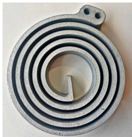
**Figure 15.** Manufactured spiral spring.
