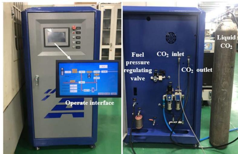
Figure 10. The scCO<sub>2</sub>-MQL cutting fluid generation device.
