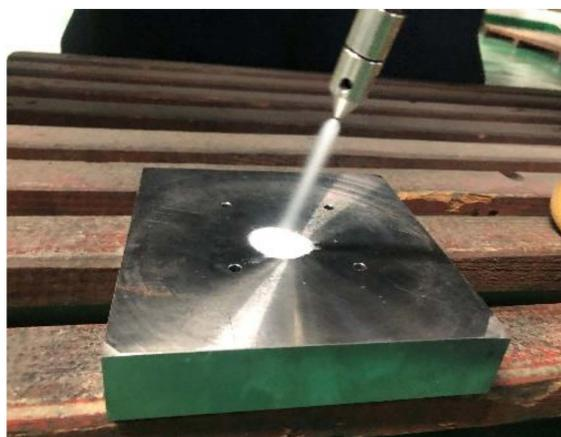
**Figure 16.** Injection of  $scCO_2$  oil into a sample.
