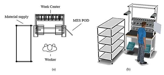
**Figure 3.** (a) Shop floor layout of the work center; (b) 3D illustration.
