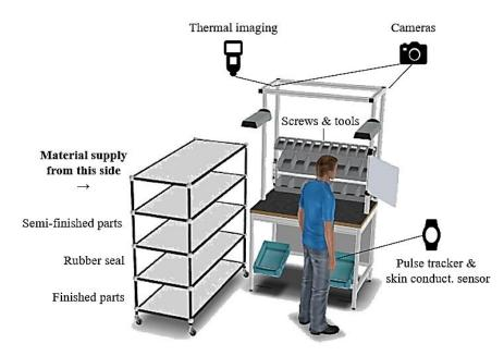
**Figure 4.** Three-dimensional illustration of the work center for the experiment including information on work instruction and measurement.
