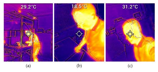
**Figure 8.** Results of different try-outs of the position for the body temperature camera: (**a**) next to the work center; (**b**) above the participant; (**c**) next to the participant.
