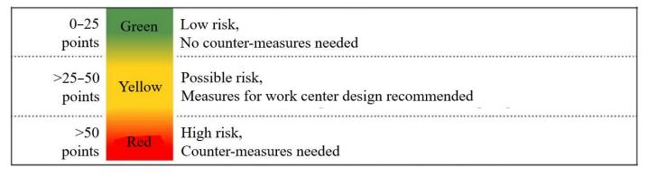
Figure 11. Ergonomic validation example from EAWS [26].
