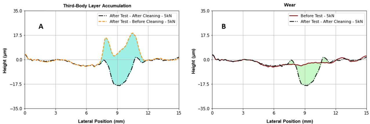
**Figure 9.** Third body layer and wear on wheel running surface after baseline tests; (A) third body layer accumulation; (B) wear.
