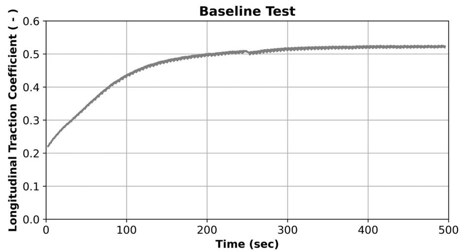
Figure 7. Longitudinal traction coefficient vs. time for baseline tests.
