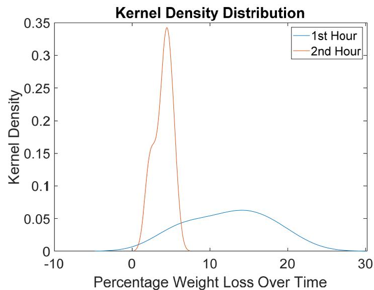
**Figure 4.** Kernel density distribution as a function of time to evaluate % weight loss during two hours.
