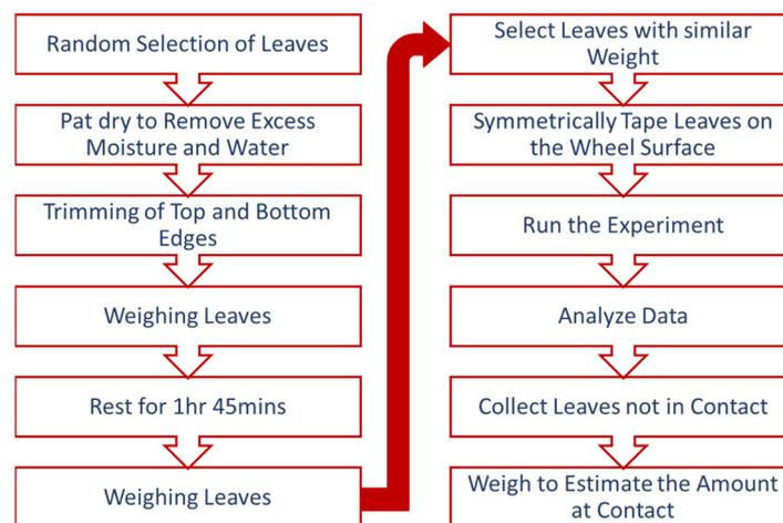
**Figure 5.** Experimental procedure flowchart.
