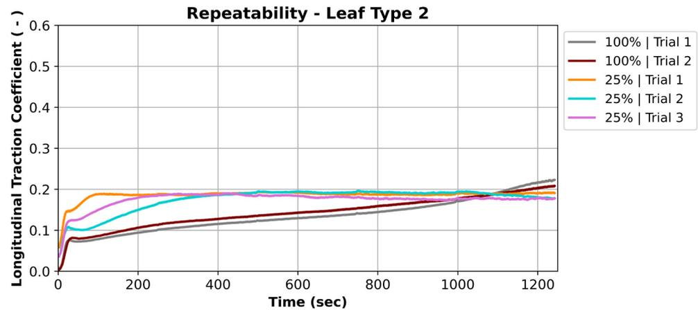
Figure 14. Repeatability tests were done with maximum and minimum categories for leaf Type 2.
