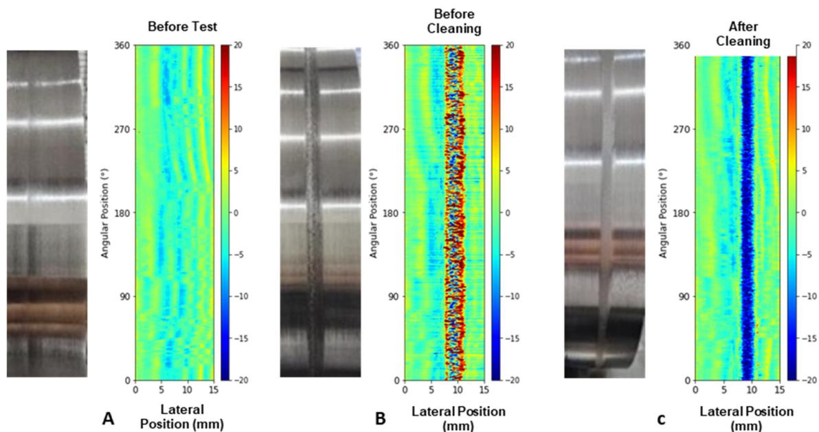
Figure 8. Wheel surface images and 2D laser measurements (A) before the test, (B) after the test with natural 3BL, and (C) after completing the test and cleaning.
