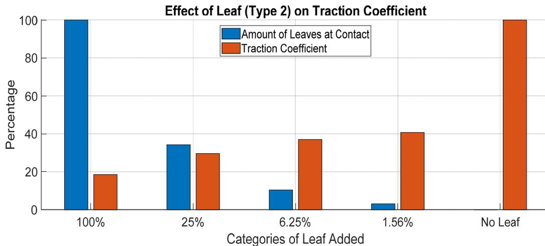
**Figure 16.** Statistical analysis on the effect of leaf Type 2 amount on traction coefficient.
