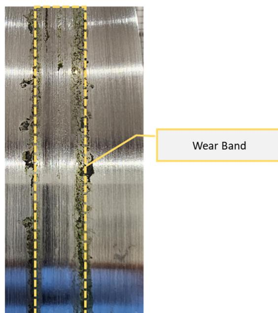
**Figure 18.** Wheel surface wear after removing leaf residues from the running surface.
