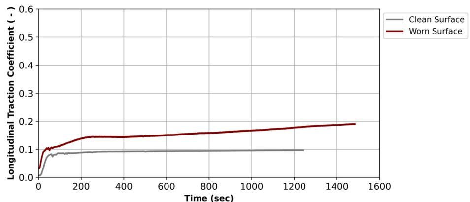
**Figure 11.** Adhesion (Longitudinal Traction Coefficient) reduction due to maximum leaf contamination when applied to a wheel with cleaned (redressed) and worn (with worn material present) surfaces.
