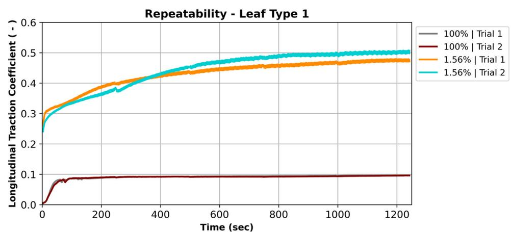
**Figure 13.** Repeatability tests for minimum and maximum amount of leaf contamination for Type 1.
