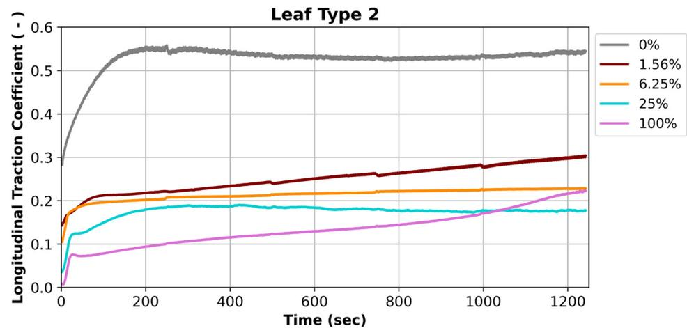
**Figure 12.** Effect of leaf volume on reducing adhesion (Longitudinal Traction Coefficient) for leaf Type 2.
