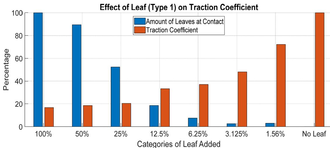
Figure 15. Statistical analysis on the effect of leaf Type 1 amount on traction coefficient.
