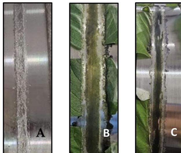
**Figure 17.** Images of wear band after (A) No Leaf, (B) 100% Leaf Type 1, and (C) 100% Leaf Type 2.
