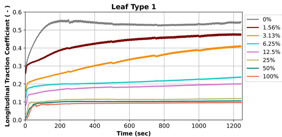
**Figure 10.** Effect of leaf volume on reducing adhesion (Longitudinal Traction Coefficient) for leaf Type 1.
