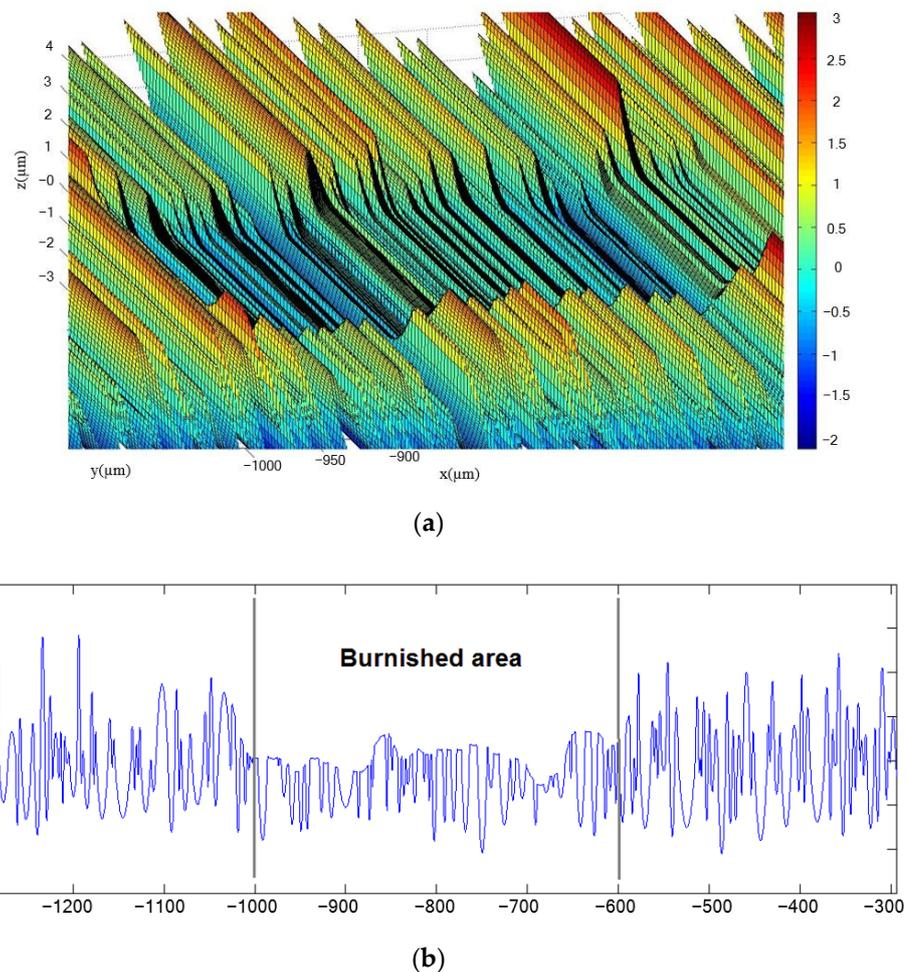
**Figure 11.** The simulated milled-burnished area (a) 3D view, (b) 2D profile (Polmax material).
