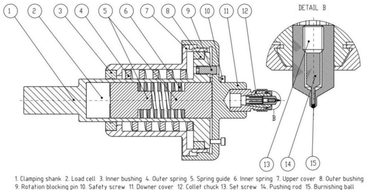
Figure 9. Design of the load cell-embedded small ball-burnishing tool.
