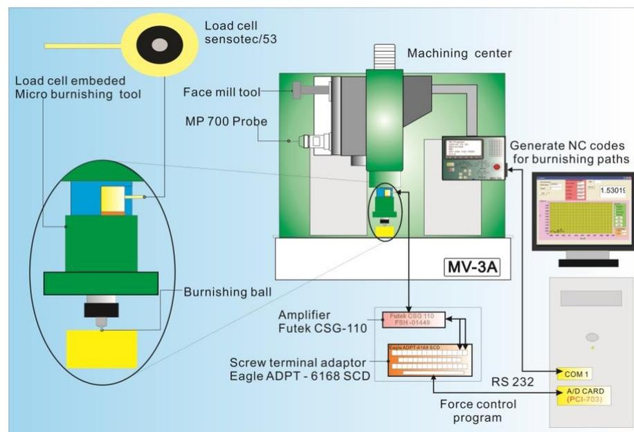
Figure 10. Experimental setup of the ball-burnishing process.
