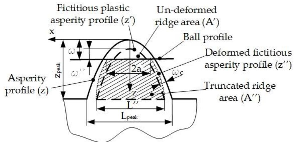
**Figure 8.** Plastic interaction between ball profile and parabolic asperity.
