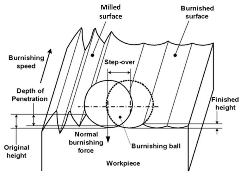
Figure 1. Schematic of the small ball-burnishing process.
