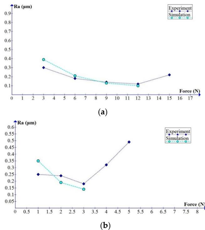
**Figure 13.** Comparison of the simulated and experimental relationships between the burnishing forces and the surface roughness: (a) Polmax and (b) on oxygen-free copper (OFC) materials.
