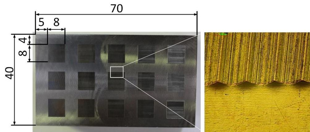
Figure 12. The experimental milled–burnished area of Polmax (optical microscope 30×).
