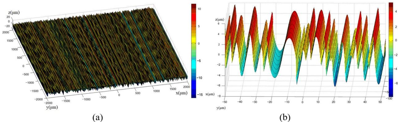
**Figure 4.** The simulated surface of the workpiece: (a)  $4000 \times 4000 \mu\text{m}$ , (b) in detail.
