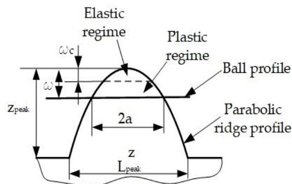
**Figure 7.** Two-dimensional elastic–plastic interaction of an individual  $\Delta y$  length parabolic ridge with a smooth surface.
