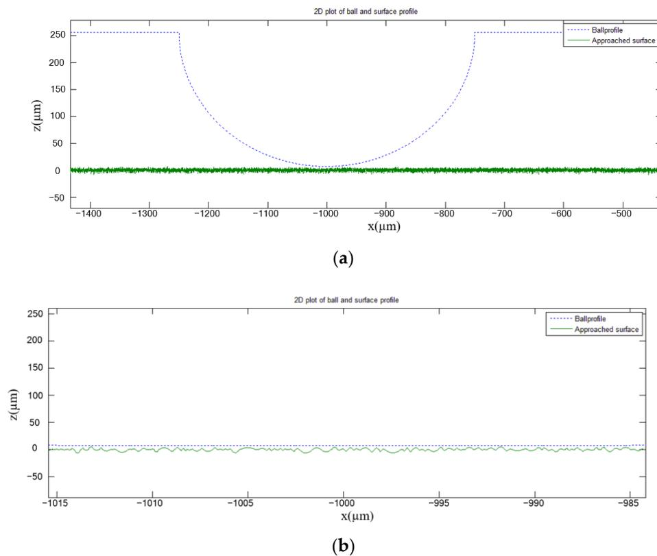
**Figure 6.** Visualization of two-dimensional contact between the ball and workpiece surfaces: (a) 1000  $\mu\text{m}$  length, and (b) in detail.
