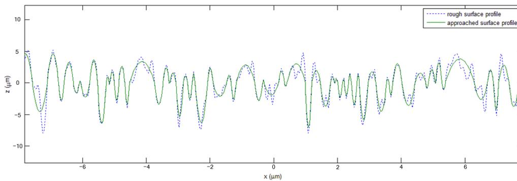
**Figure 3.** Aramaki's roughness approximation.
