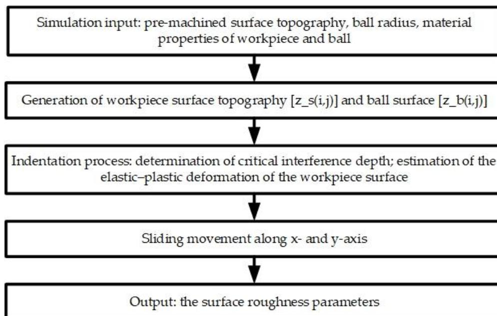
Figure 2. Simulation procedure of the smoothing small ball-burnishing process.
