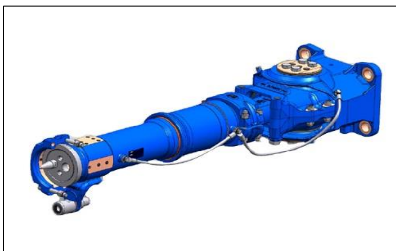
Figure 3. Intermediate coupler (rubber buffer and deformation tube) [12].
