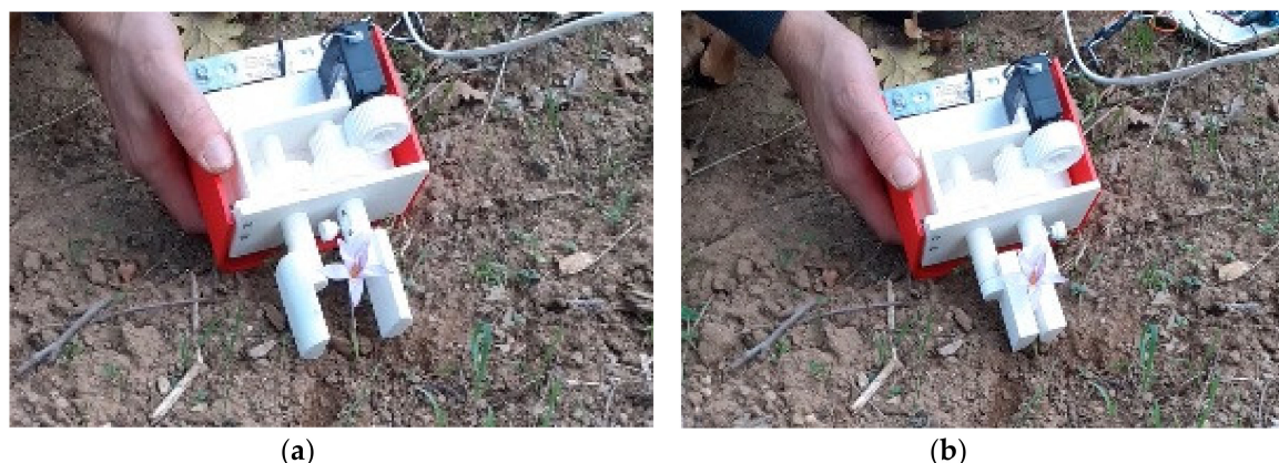
Figure 20. Field tests on wild saffron flowers: (a) approaching the flower; (b) harvesting phase.
