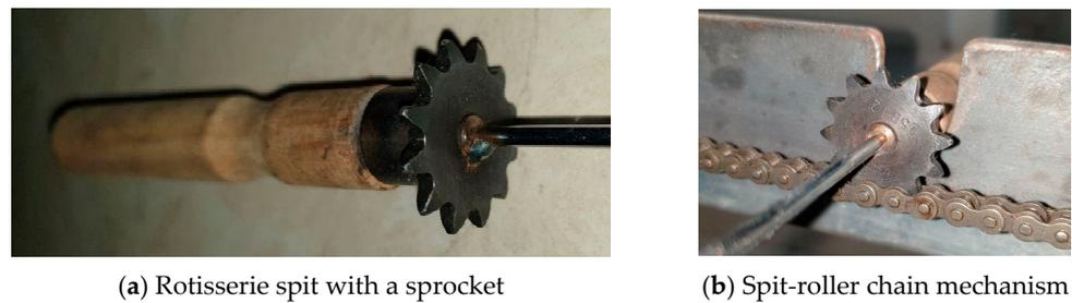
**Figure 8.** The rotisserie spit used for the spit-roller chain engagement.
