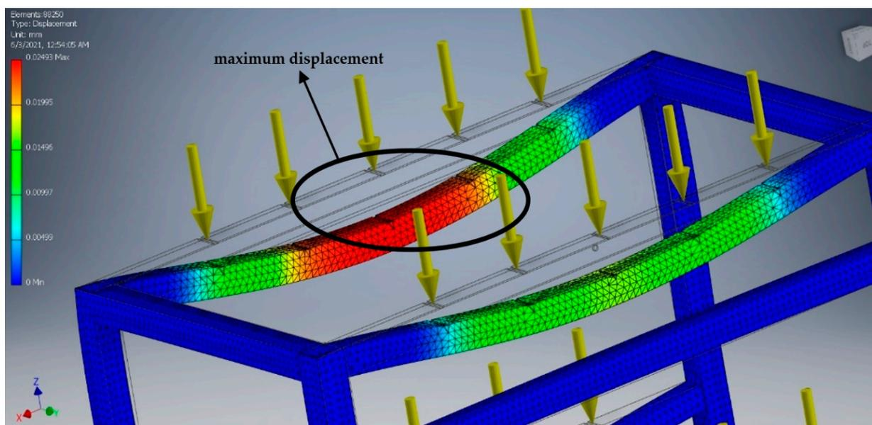
**Figure 2.** Stress simulation results for the frame (displacement).
