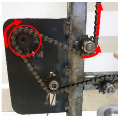
(c) Sprocket configuration on the motor bracket
