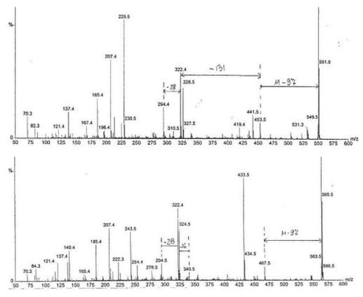
**Figure 6.** MS/MS spectra (electro spray +1) of the methyl analogues: above with molecular ion m/z **550**, showing loss of 97, 131 and 28 mass units equal to proline, methionine and 2xCH<sub>2</sub>, respectively; below with molecular ion m/z **564**, showing loss of 97, 16 and 28 mass units equal to proline, NH<sub>2</sub> and 2 CH<sub>2</sub>, respectively.
