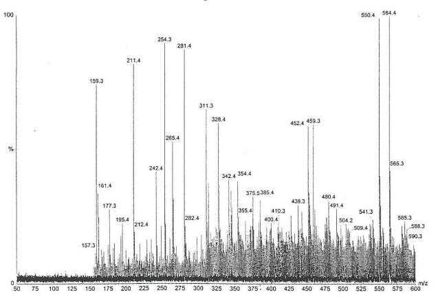
**Figure 5.** Mass spectrum (electro spray +1) of the sub-fraction of Fraction 2, showing the prominent pair of methyl analogues m/z 550 and m/z 564.
