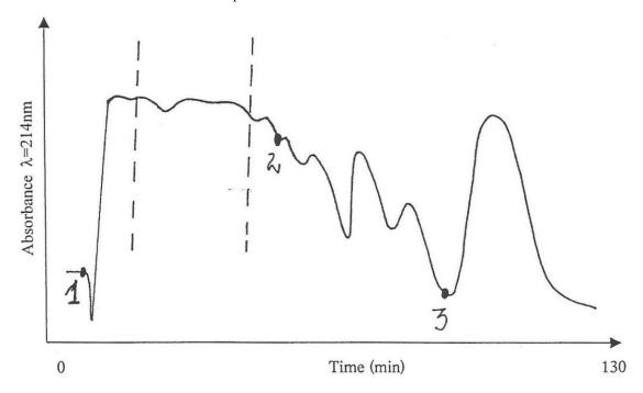
**Figure 4.** Absorbance pattern of the water-soluble fraction and its fragmentation into 3 sub-fractions obtained by isocratic (50% acetonitrile in water) MPLC. Numbers indicate the point at which each fraction commences.
