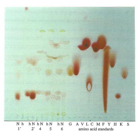
**Figure 3.** Silica gel chromatography of samples of fermentation Fractions 1', 2', 4, 5 and 6 (N) compared with hydrolysed aliquots (h) of the same, and with reference to some amino acid standards. Sprayed with ninhydrin reagent. Note the yellow high Rf value spot, each for hydrolysed Fractions 4–6, attributed to proline.
