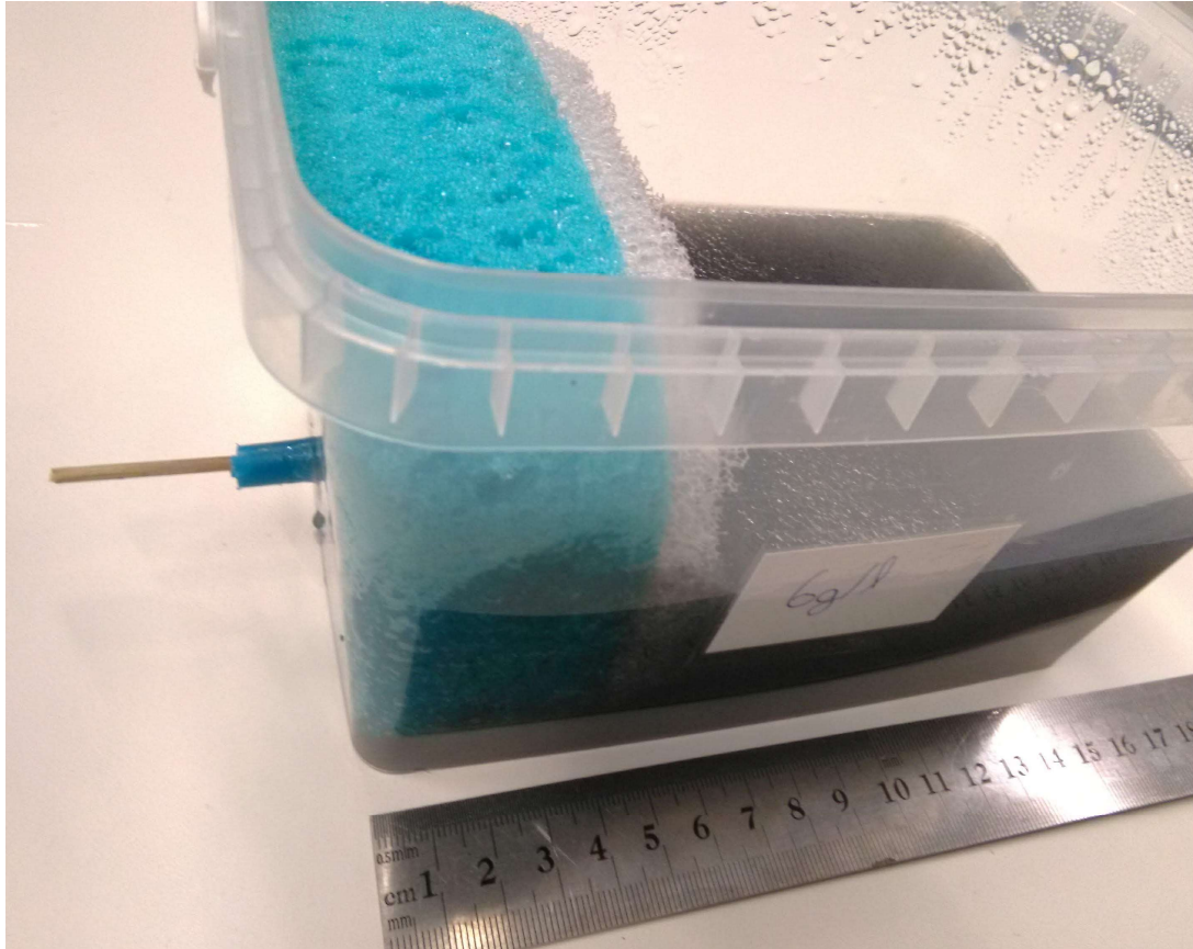
Figure S2. The photo of prepared TMM in the container. Wooden rod (2 mm in diameter) was embedded for more than 9 cm in the TMM trough sidewall of container. The rod was actuated linearly by push-pull motion from solenoid, excited at defined frequency and voltage amplitude from geerator.
