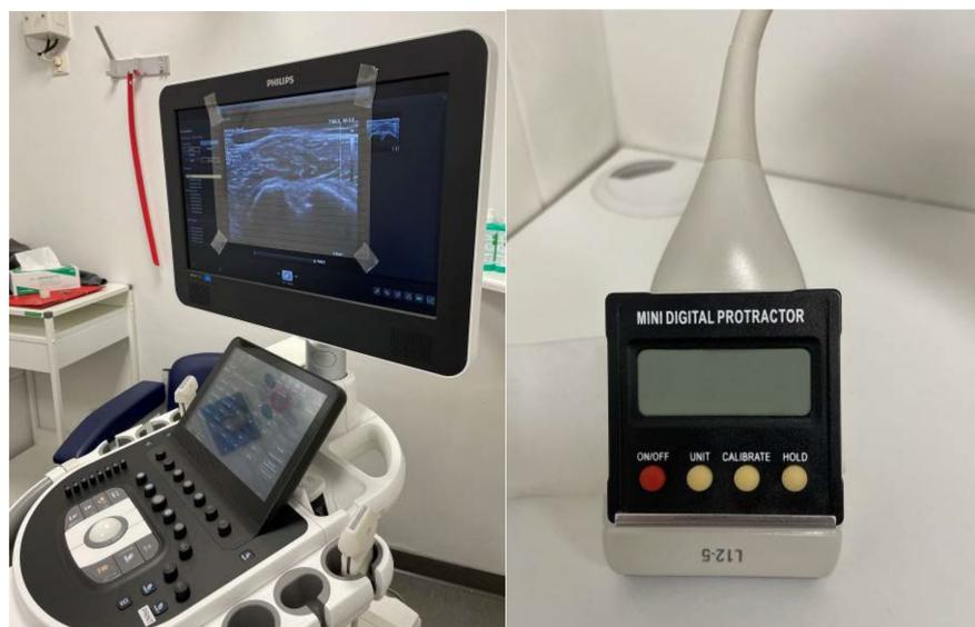
**Figure 1.** Equipment for sonographically assisted measurement of humeral torsion.
