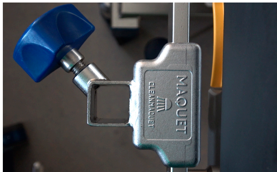
Figure 6. In version B, fixation takes place via a common square tube holder (Maquet GmbH, Rastatt, Germany).
