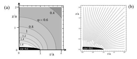
**Figure 4.** Newtonian attraction to a highly flattened constant density oblate spheroid (black shape) with a 1:10 axial ratio similar to those of spiral galaxies. One quadrant is shown: (**a**) contour plot of the Newtonian gravitational potential exterior to the oblate, shown in units of *GMm/a*; (**b**) lines of exterior force. Reprinted from Figure 7e,f in Reference [58], with permission from Elsevier.
