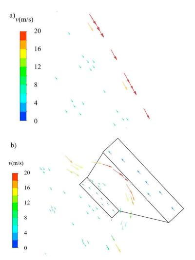
Figure 9. Velocity vectors of fluid in different blades. (a) Smooth blade; (b) Bionic blade.
