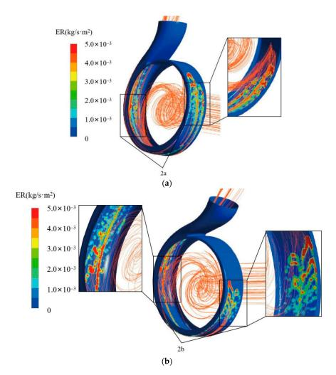
**Figure 11.** Cloud diagram of volute particle trajectory and wear rate for two different blades. (a) Smooth blade; (b) Bionic blade.
