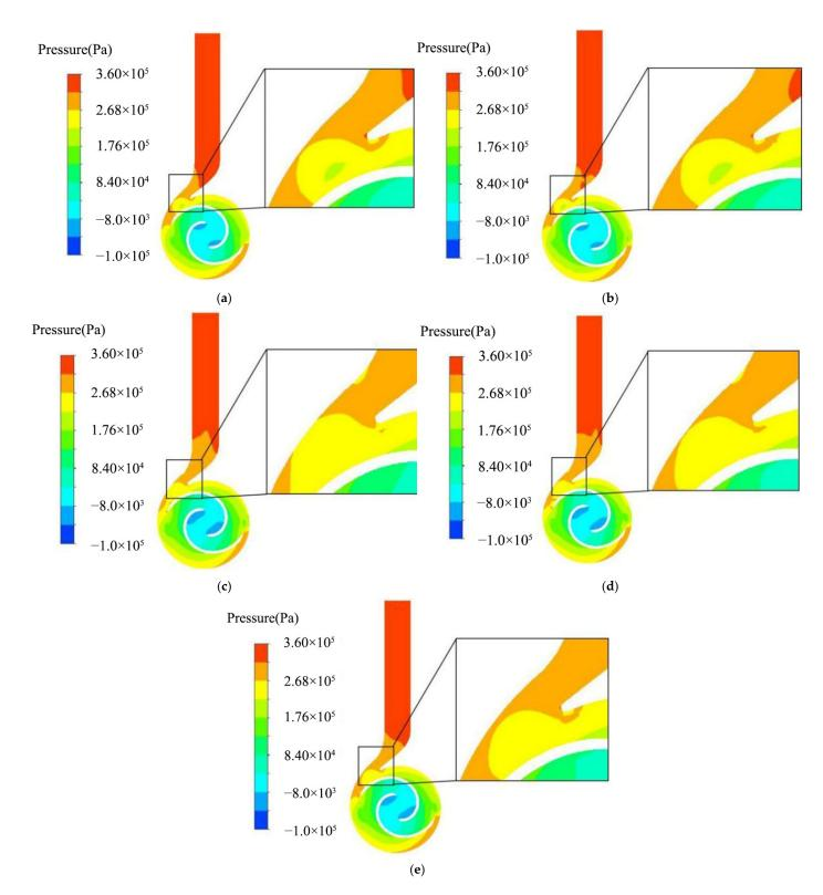
**Figure 4.** Pressure cloud diagram of pump sections with different blades. (a) Smooth blades; (b) h = 3 mm; (c) h = 5 mm; (d) h = 7 mm; (e) h = 9 mm.
