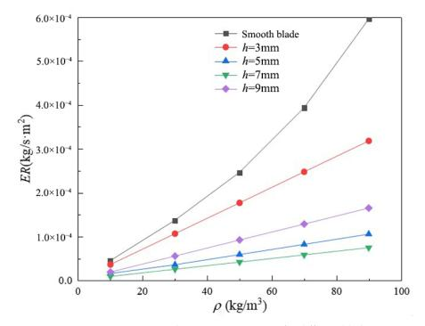
Figure 6. Average wear rate-particle concentration curve for different blade pumps.
