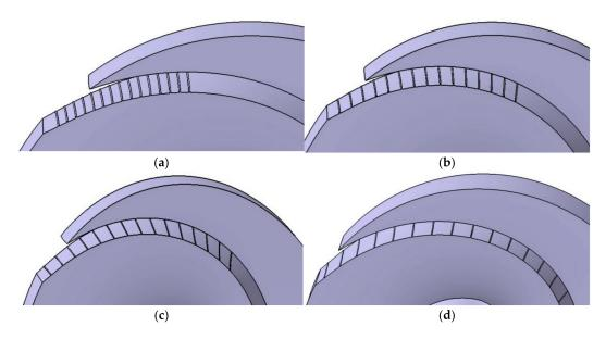
**Figure 2.** Fluid domain of the impeller of a bionic blade with different groove spacing. (a) h = 3 mm; (b) h = 5 mm; (c) h = 7 mm; (d) h = 9 mm.
