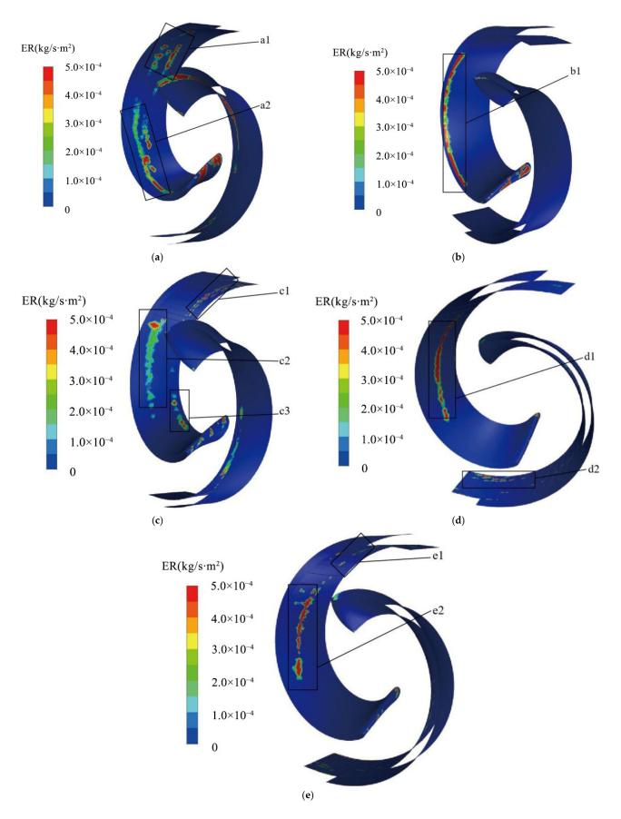
**Figure 8.** Wear cloud diagram of a smooth blade and four different bionic blades. (a) Smooth blades; (b) h = 3 mm; (c) h = 5 mm; (d) h = 7 mm; (e) h = 9 mm.
