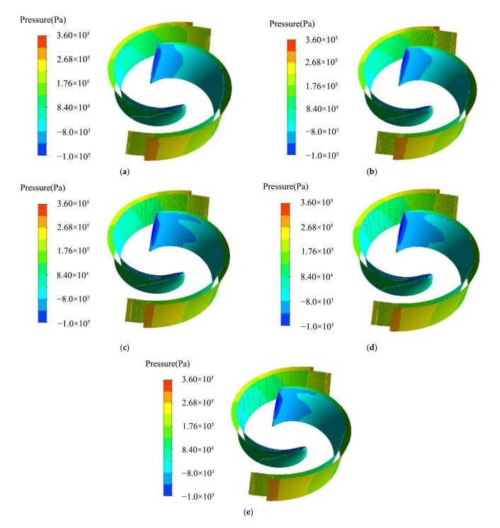
**Figure 5.** Cloud diagram of blade pressure distribution at different blades. (a) Smooth blades; (b) h = 3 mm; (c) h = 5 mm; (d) h = 7 mm; (e) h = 9 mm.
