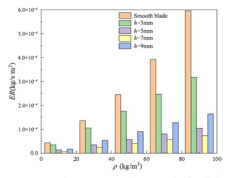
Figure 7. Histogram of average wear rate-particle concentration for different blade pumps.
