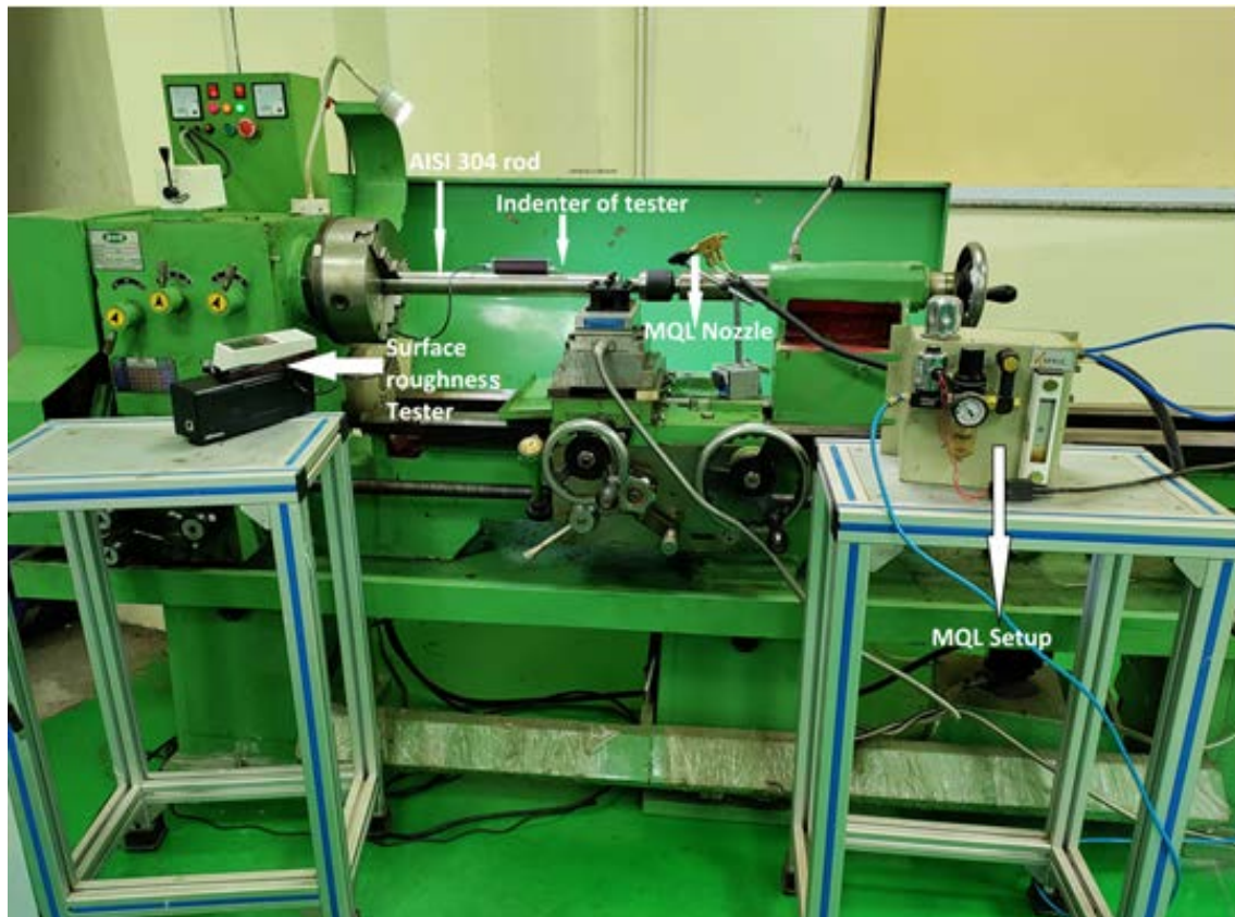
Figure 1. Experimental setup for turning of AISI 304 steel.
