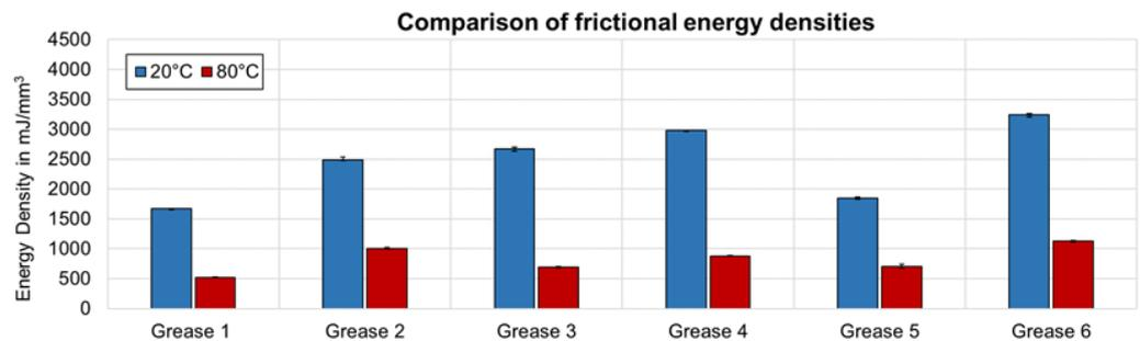
Figure 5. Energy densities,  $e_{\text{Rheo}}$ , of all greases at 20 and 80 °C.
