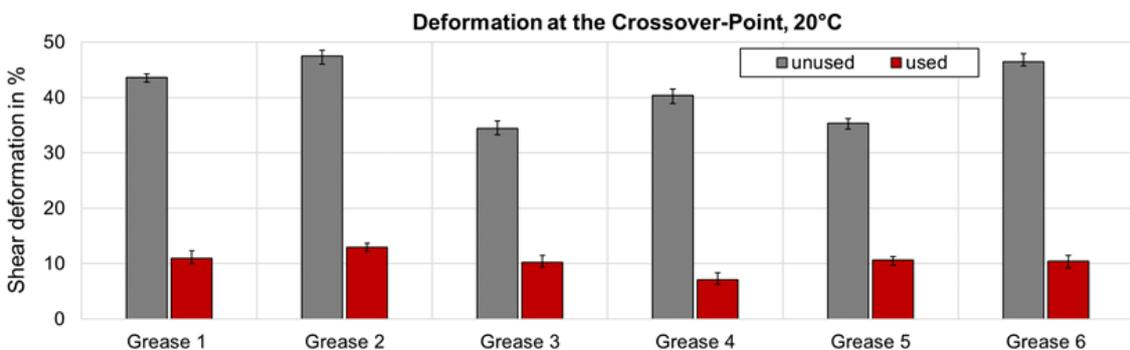
Figure 23. Comparison of deformations at the crossover point for unused and used greases.
