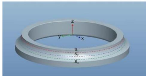
**Figure 2.** Schematic representation of three scanning paths ( $s_1$ ,  $s_2$ , and  $s_3$ ) for damage's depth measurement.
