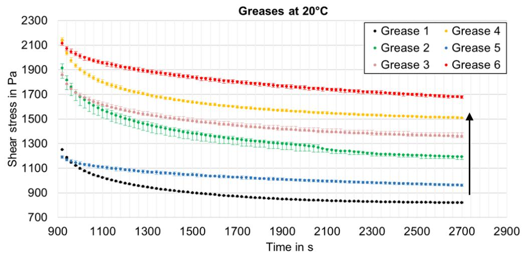
Figure 4. Transient flow curves of all greases at 20 °C.
