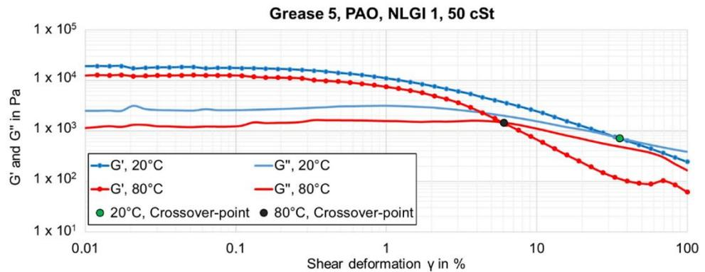
Figure 8. Measurement curves from amplitude test for Grease 5.
