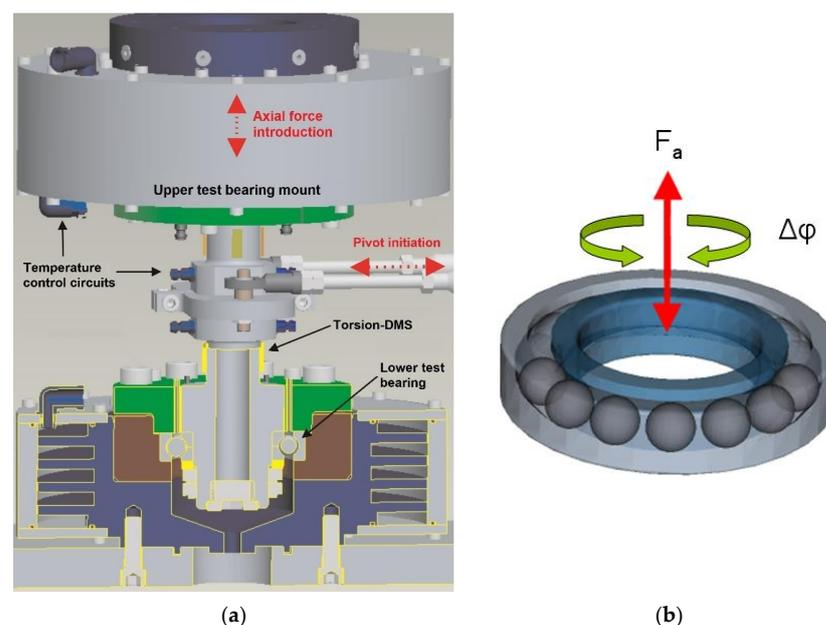
**Figure 1.** Schematic view of ITR-Roller-Bearing Test (a); test-arrangement, movement, and load direction four-point angular contact ball bearing (b).
