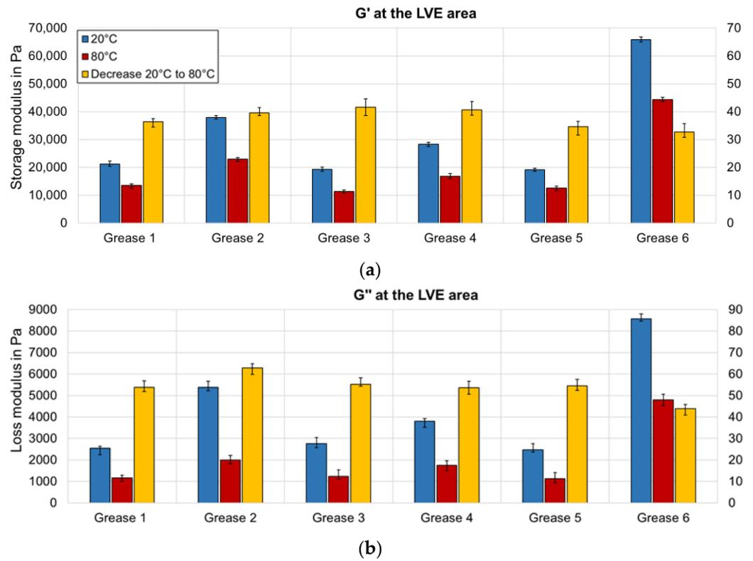
Figure 6. Storage (a) and loss (b) moduli within LVE range.
