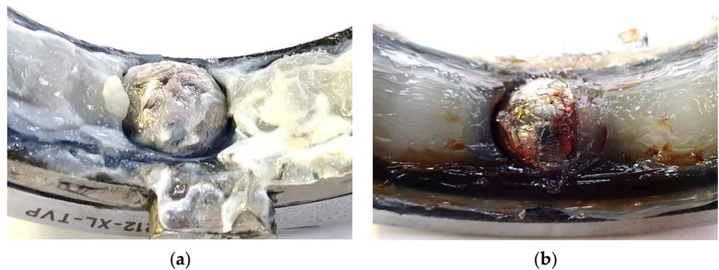
**Figure 18.** Fat sample Grease 4 at the beginning of test (a) and after end of the test (b) (detailed image of steel ball bearing).
