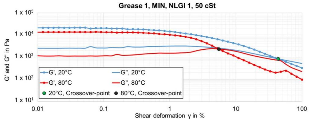
Figure 7. Measurement curves from amplitude test for Grease 1.
