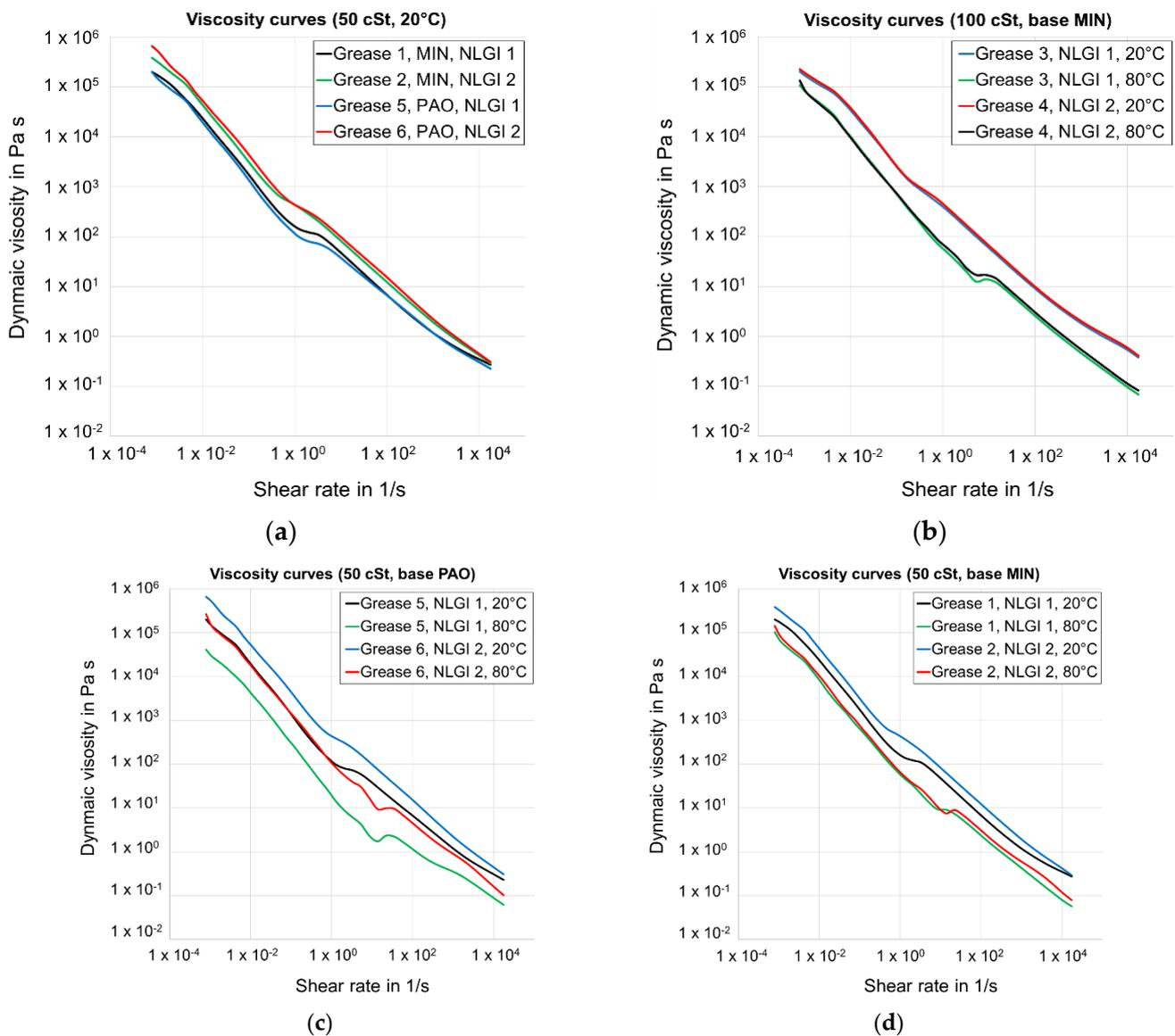
**Figure 3.** Viscosity shear rate behavior (base oil viscosity, 50 cSt (a) and 100 cSt (b)): temperature effect on viscosity for synthetic-oil-based (c) and mineral-oil-based (d) lubricating greases.
