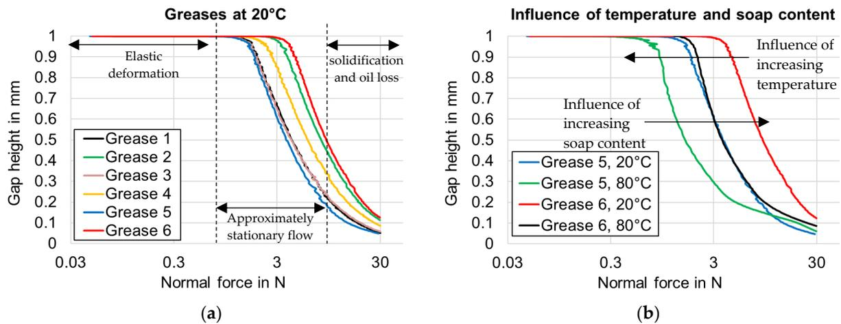
Figure 13. Comparison of all greases at 20 °C (a); influence of temperature and soap content on forming work (b).
