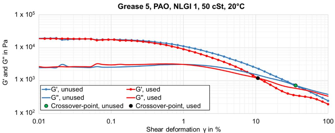
Figure 22. Comparison of unused and used Grease 5.
