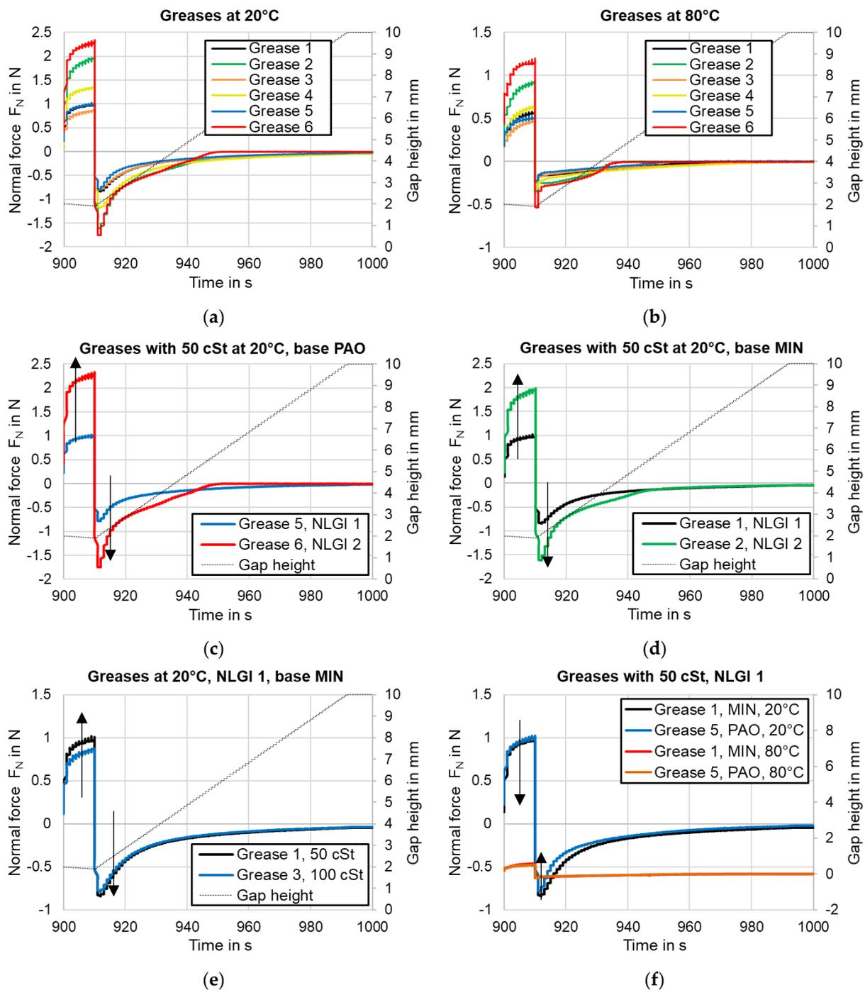
**Figure 10.** Results for greases at 20 °C (a) and 80 °C (b). Influence of soap content on tackiness of synthetic-oil-based (c) and mineral-oil-based (d) grease. Influence of base oil viscosity on tackiness. (e) Influence of temperature on tackiness (f).
