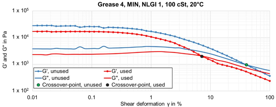
Figure 21. Comparison of unused and used Grease 4.
