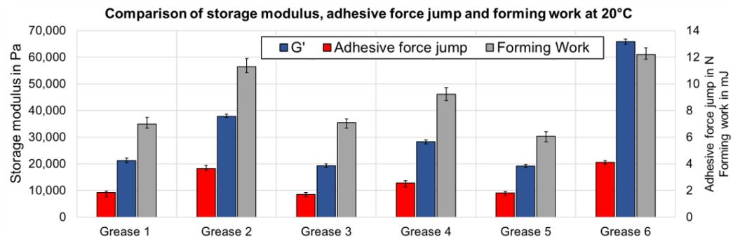
Figure 15. Comparison of storage modulus, adhesive force jump, and forming work.
