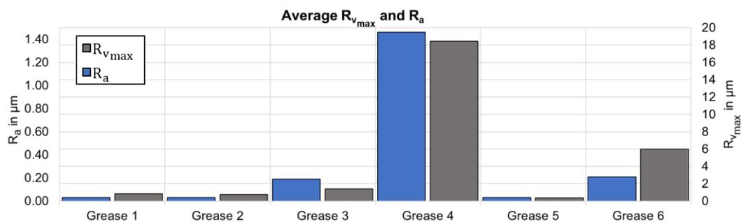
**Figure 19.** Average depth of damage.
