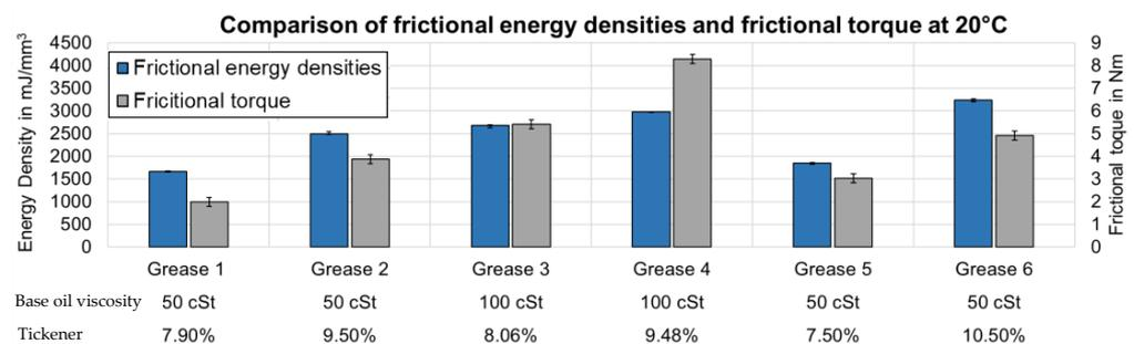
Figure 17. Comparison of frictional energy densities and frictional torque.
