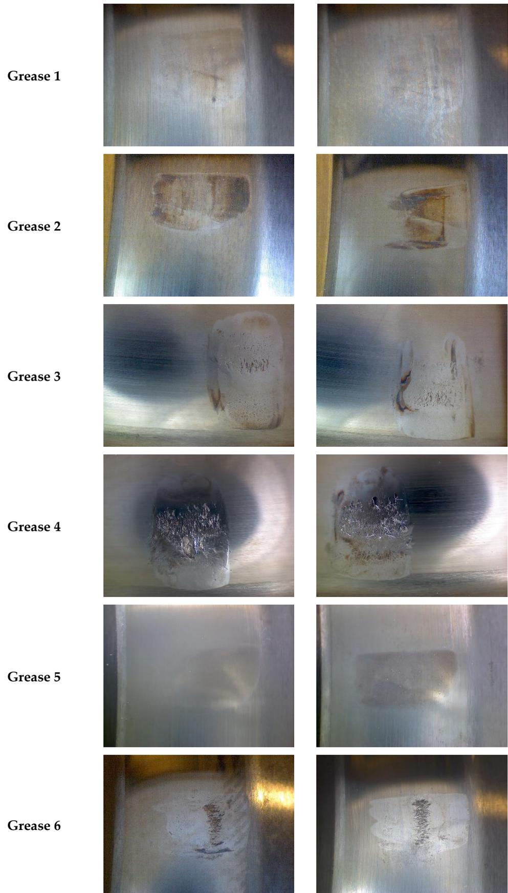
**Figure 20.** Damages in rolling bearings with various greases (right column shows each failure of lower ring).
