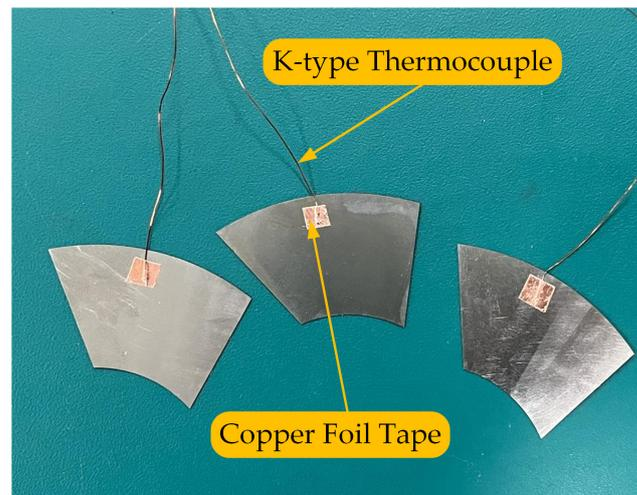
**Figure 13.** Temperature measurement points layout of the top foils.
