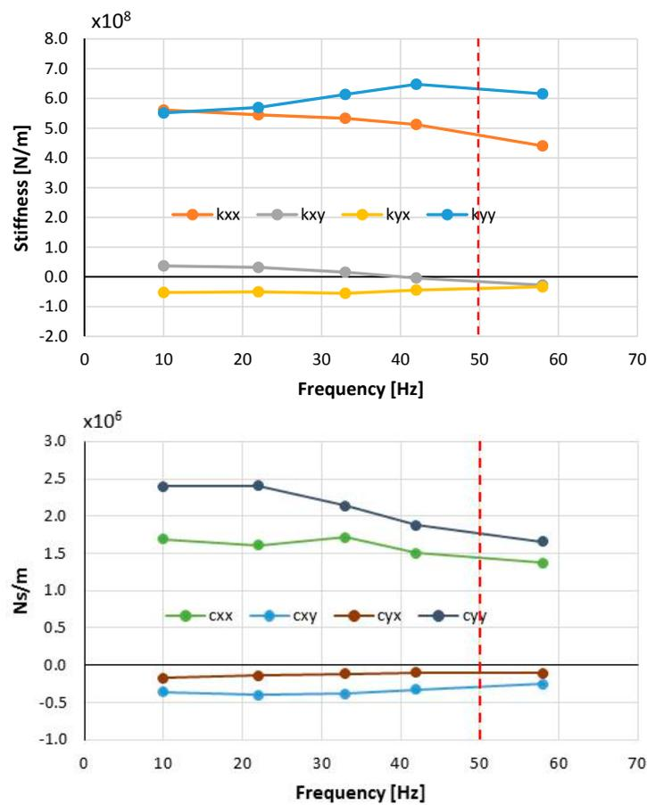
Figure 15. Stiffness and damping coefficients as function of excitation frequency, at 3000 rpm (50 Hz) rotational speed, for a load of 58 kN (y: vertical direction, x: horizontal direction, the dashed red vertical line indicates the rotational frequency).
