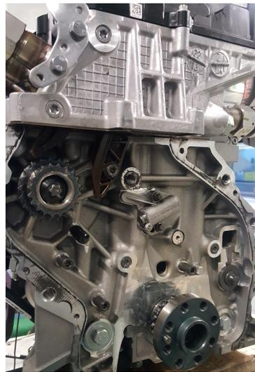
Figure 12. The deactivated timing drive system.
