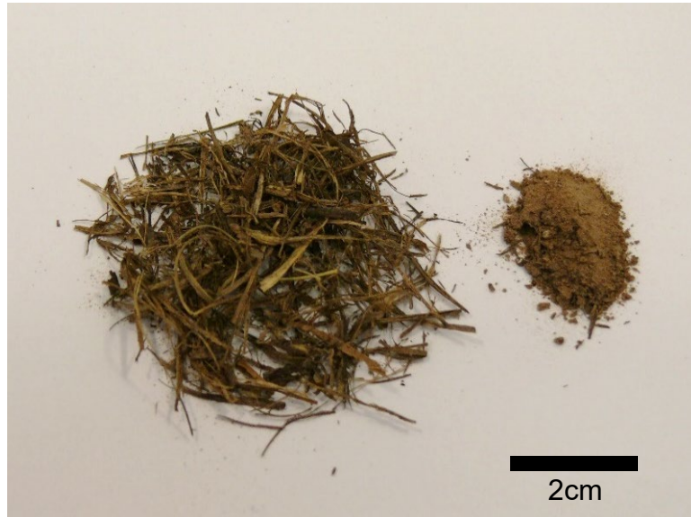
Figure S1: Example of the building materials used for the construction of a single turret. One original turret was first dissolved in demineralized water, and thereafter its components separated into plant (mostly grass blades) and soil materials, and dried overnight at 50°C to quantify their mass.
