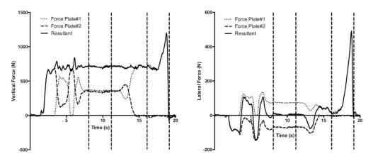
**Figure 1.** Vertical (**left** panel) and lateral (**right** panel) forces during a single-leg, medial countermovement jump from a representative trial. The three traces represent force plate #1 (dotted line), force plate #2 (dashed line) and resultant force (solid line). From left to right on each panel, the four vertical dashed lines reflect the beginning and end of standing prior to the jump, the initiation of jump (lateral forces >10 N) and end of jump.
