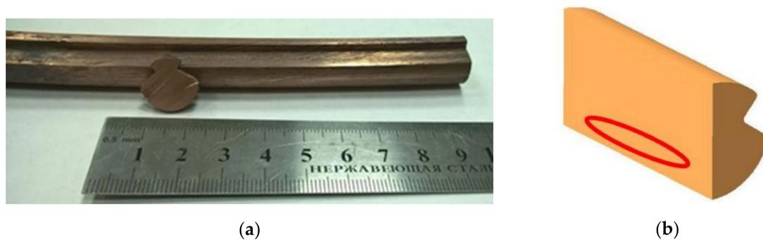
**Figure 4.** Laboratory samples after ECAP with wire forming (a) and area for microstructural analysis (b).
