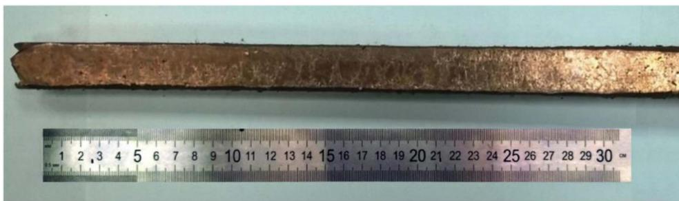
**Figure 1.** Laboratory samples after radial swaging with a degree of accumulated strain of  $e = 1.5$ .
