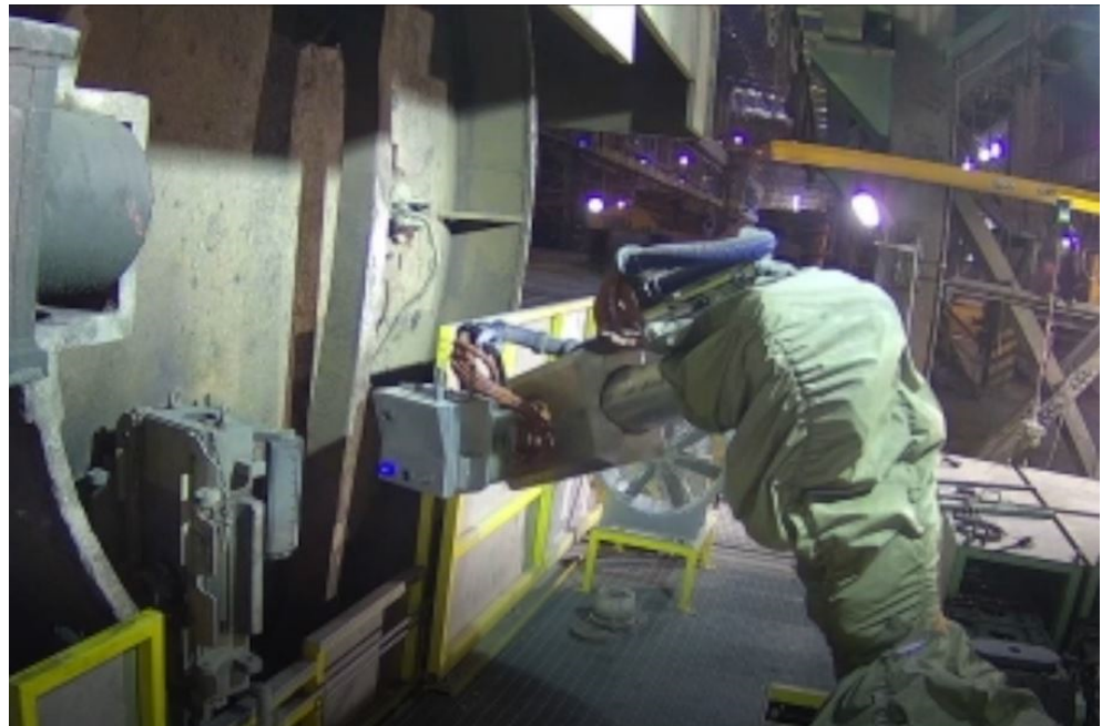
Figure 4. The robot inspects the opened sliding gate by means of the vision tool.
