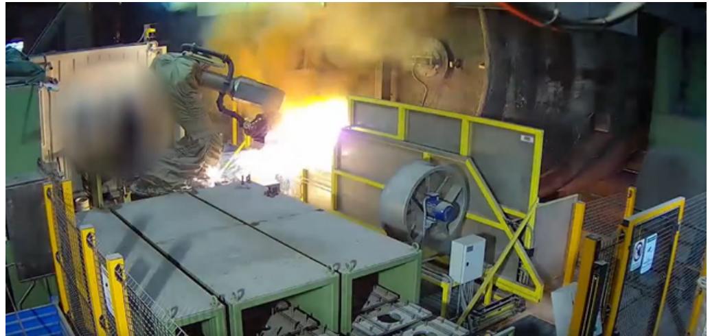
Figure 11. The robot opens the tap hole using an oxygen lance.
