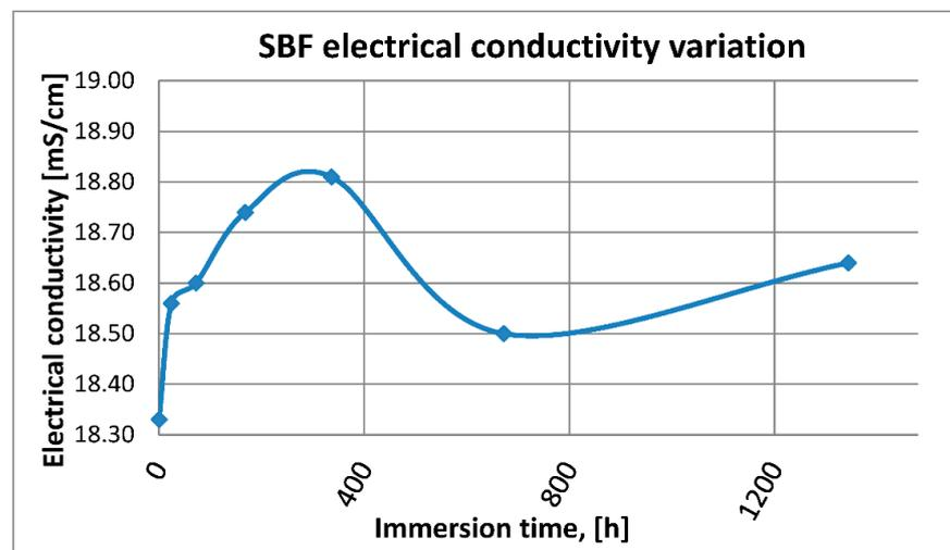
Figure 5. SBF electrical conductivity vs. immersion time variation.
