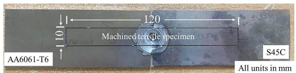
**Figure 2.** Dimensions for a tensile specimen from a butt FSSW joint.
