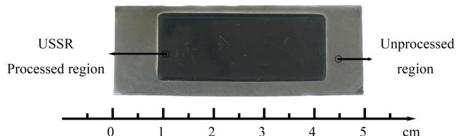
**Figure 1.** Appearance of the sample after USSR processing.
