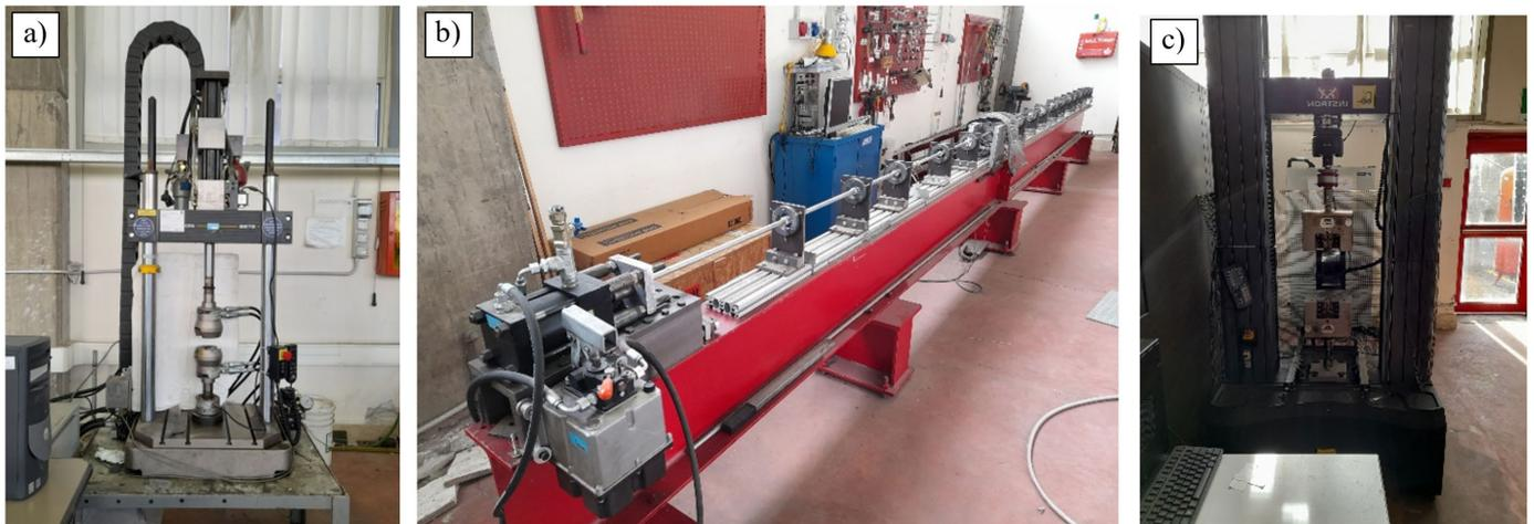
**Figure 2.** Testing equipment for experiments: (a) Hydraulic machine for slower dynamic tests, (b) SHTB for faster dynamic tests, and (c) motor-driven machine with climatic chamber for static tests at different temperatures.
