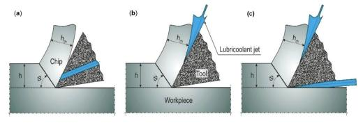
**Figure 4.** The methods of supplying a lubricating medium to the work–tool interface, inserted from: (a) from the side of the rake face; (b) on the rake face; (c) on the flank and rake face [39].
