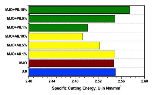
**Figure 6.** The variation of the specific cutting energy with respect to the mixture of modified jatropha oil (MJO) and AIL/PIL [66].
