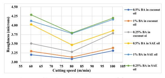
Figure 7. The variation of the surface roughness with the cutting speed [67].
