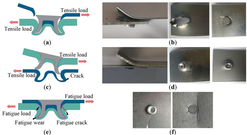
**Figure 3.** (a) Tensile failure mode of SA joint; (b) tensile failures of SA joint; (c) tensile failure mode of AS joint; (d) tensile failures of AS joint; (e) fatigue failure mode; (f) fatigue failures of joints.
