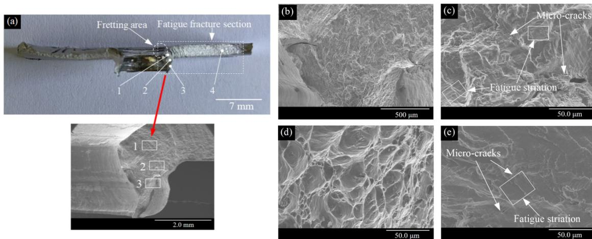
**Figure 14.** Fatigue fracture micro-morphology of AA5052 sheet in the SA joint. (a) Macroscopic morphology of the fatigue fracture; (b) magnified morphology of area 1; (c) micro-morphology of area 2; (d) micro-morphology of area 3; (e) micro-morphology of area 4.
