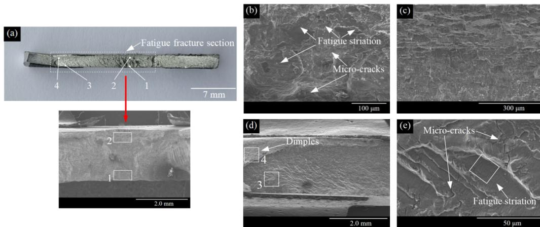
**Figure 15.** Fatigue fracture micro-morphology of AA5052 sheet in the AS joint. (a) Macroscopic morphology of fatigue fracture; (b) micro-morphology of area 1; (c) micro-morphology of area 2; (d) micro-morphology of areas 3 and 4; (e) magnified morphology of area 3.
