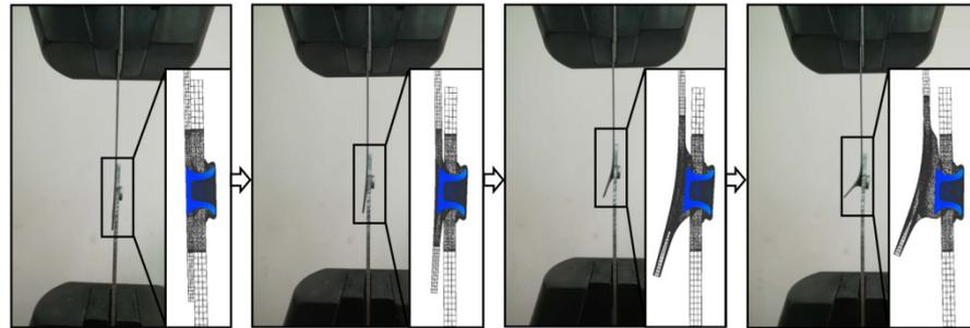
Figure 7. The tensile test process of the SA joint.
