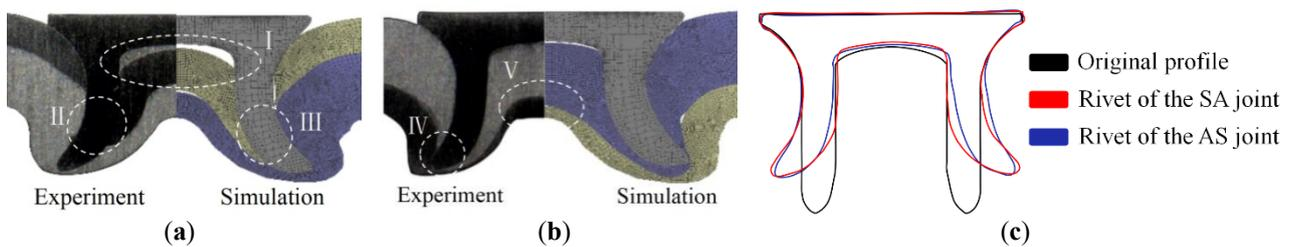
**Figure 5.** Section profile comparison. (a) Experiment section and simulation section of the SA joint; (b) experiment section and simulation section of the AS joint; (c) original profile and deformed profiles of rivets.
