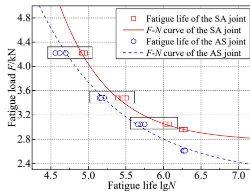
**Figure 10.**  $F$ - $N$  curves of the SA joint and the AS joint.
