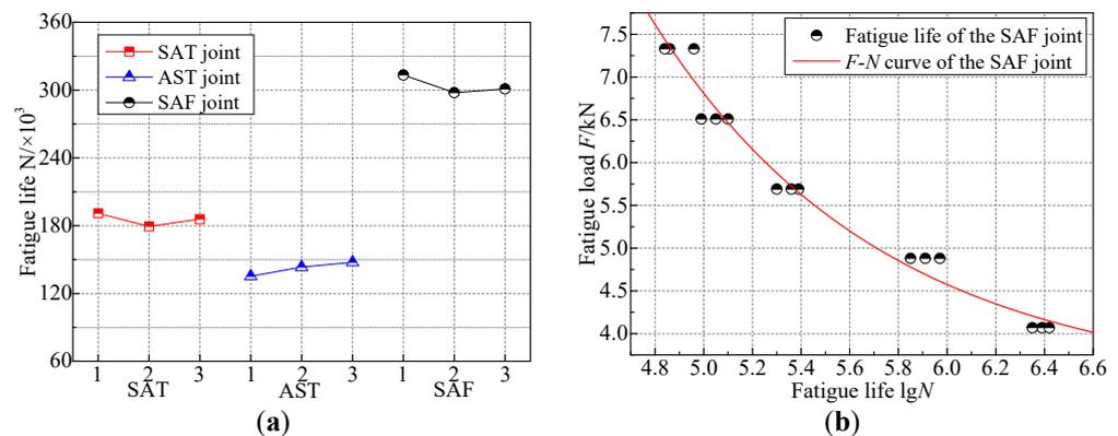
**Figure 11.** The fatigue life of two-rievt joints. (a) A comparison of two-rievt joints; (b)  $F-N$  curve of the SAF joint.
