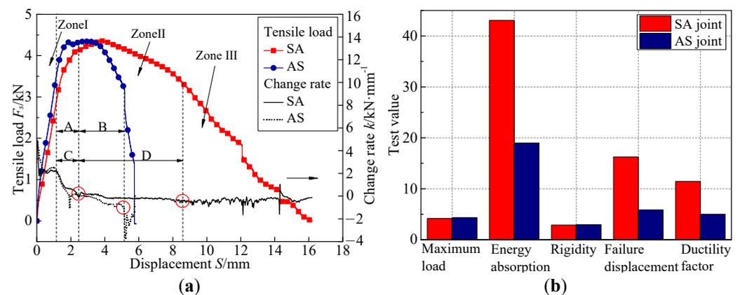
Figure 8. Tensile property of single-rivet joints. (a)  $F_s$ - $S$  curves and  $k$ - $S$  curves; (b) test values.
