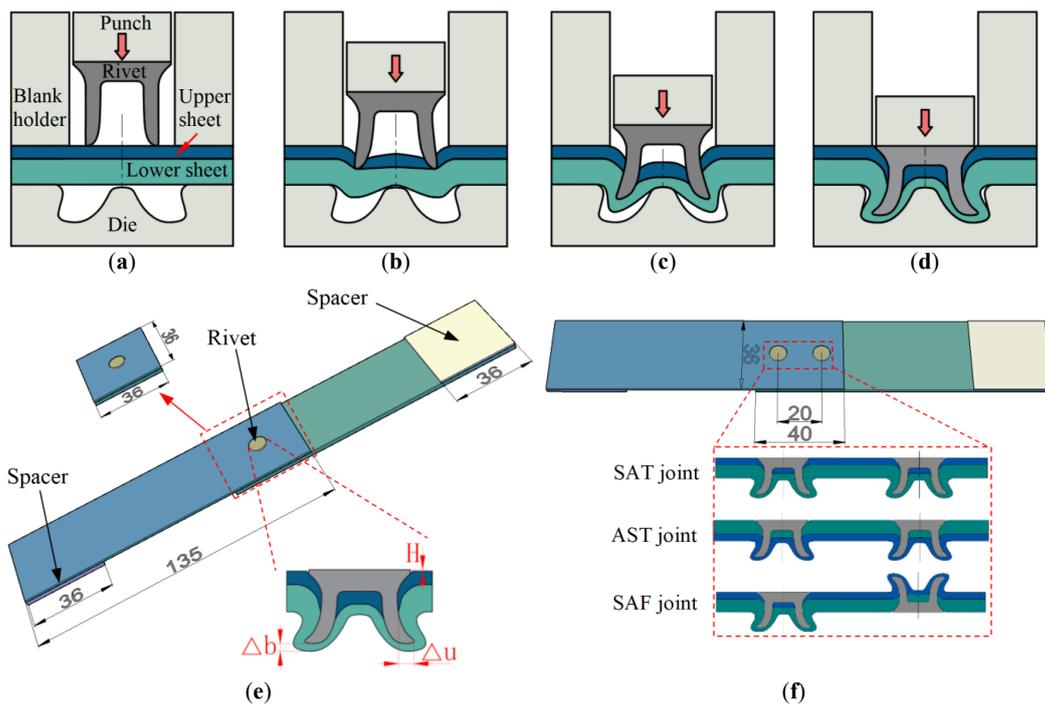
**Figure 2.** Forming process and geometry sizes of the SPR specimen. (a) Clamping; (b) puncture; (c) expansion; (d) forming; (e) single-rivet joint; (f) two-rivet joint (unit: mm).
