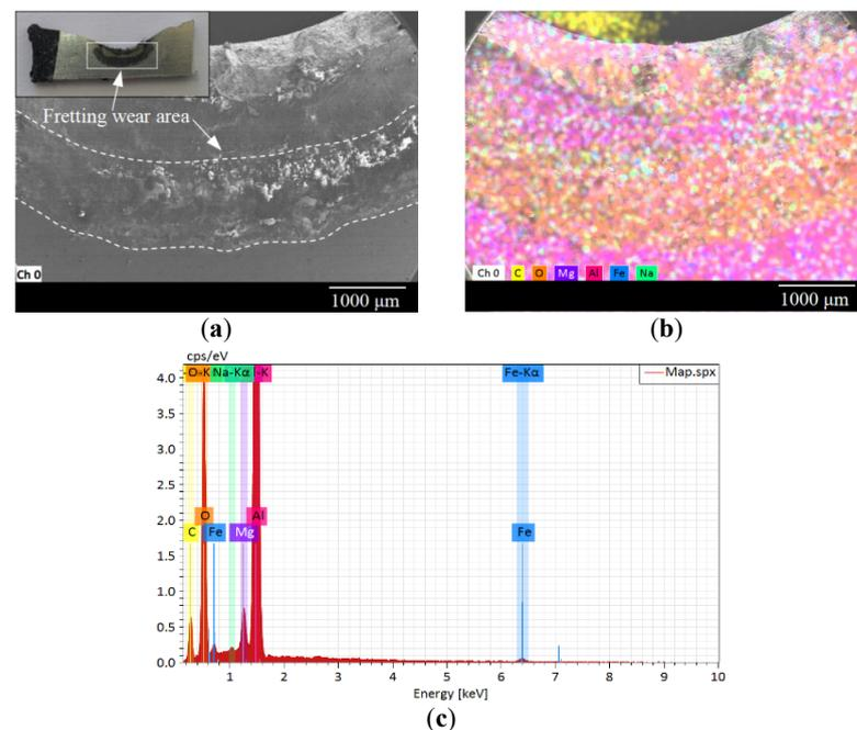
**Figure 16.** Morphology of contact interface between sheets. (a) Morphology of contact interface; (b) element composition; (c) mass fraction of the elements.
