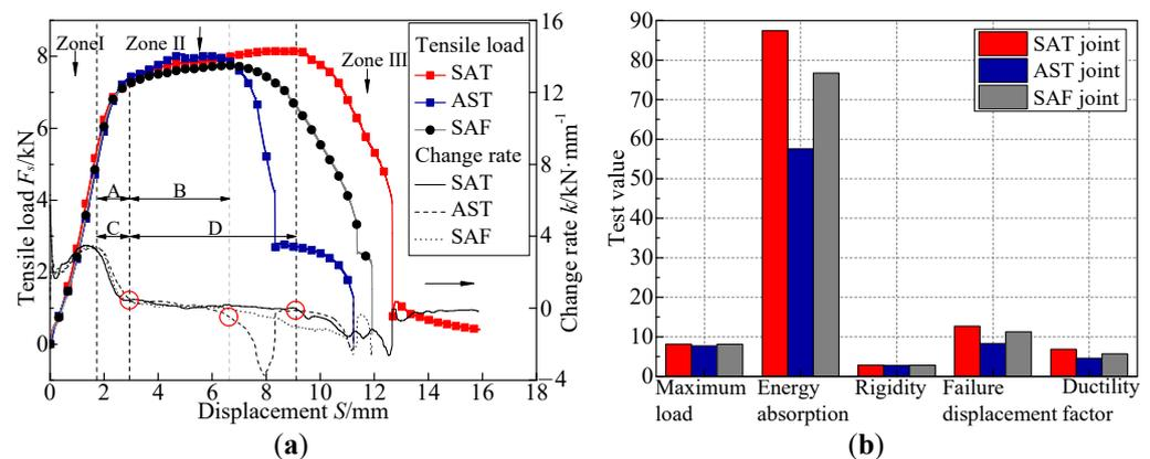
**Figure 9.** Tensile property of two-rivet joints. (a)  $F_s$ - $S$  curves and  $k$ - $S$  curves; (b) test values.
