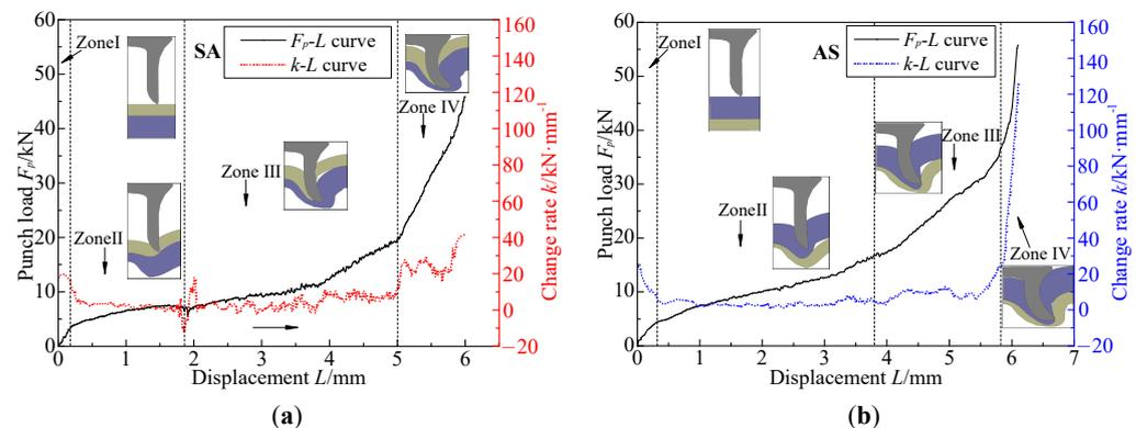
**Figure 4.** The  $F_p$ - $L$  curve and  $k$ - $L$  curve of (a) the SA joint and (b) AS joint.
