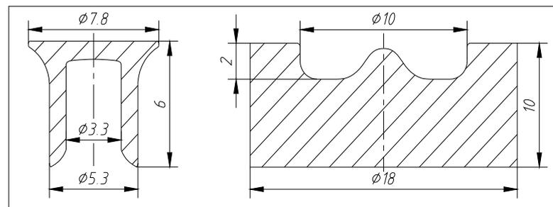
**Figure 1.** Geometry and sizes of the rivet and die (Unit: mm).
