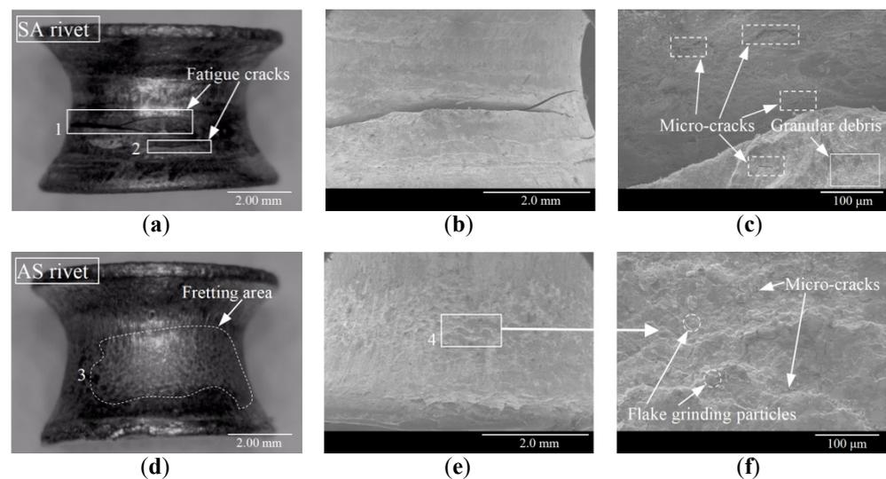
**Figure 13.** Micro-morphologies of the SA rivet and AS rivet. (a) SA rivet; (b) cracks of area 1; (c) micro-cracks of area 2; (d) AS rivet; (e) fretting wear of area 3; (f) micro-cracks of area 4.
