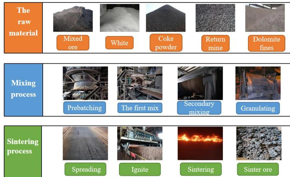
**Figure 2.** Sintering Metallogensis process of iron ore powder.
