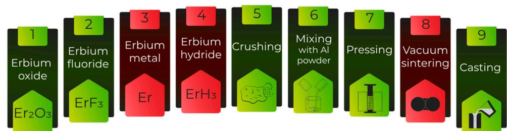
**Figure 1.** Two methods of obtaining erbium alloys: alloying using the hydrogenation technology RZM (1–9) or dispersion strengthening with ErF<sub>3</sub> particles (1, 2→5–7→9).
