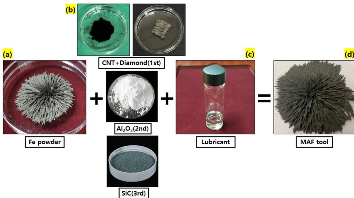
**Figure 5.** Images of a mixture of magnetic abrasive tools: (a) Fe powder; (b) CNT + diamond paste (1st),  $\text{Al}_2\text{O}_3$  (2nd), and SiC (3rd); (c) lubricant, and (d) their mixture to produce an MAF tool.
