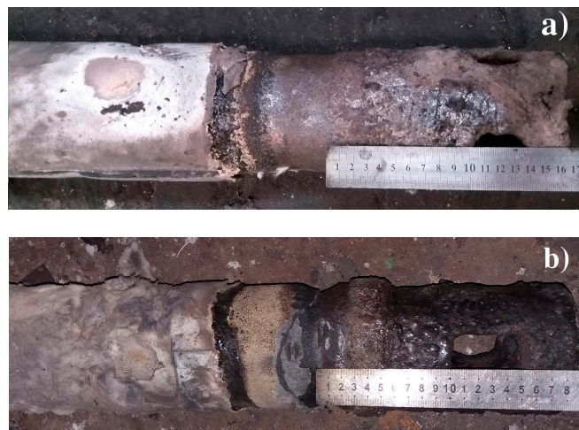
Figure 10. Comparison between the external wall topographies of the used SFN (a) and bilateral-port nozzle (b) after a sequence casting period.
