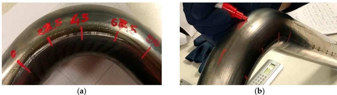
**Figure 16.** Thicknesses measuring grid on the backbone (a,b).
