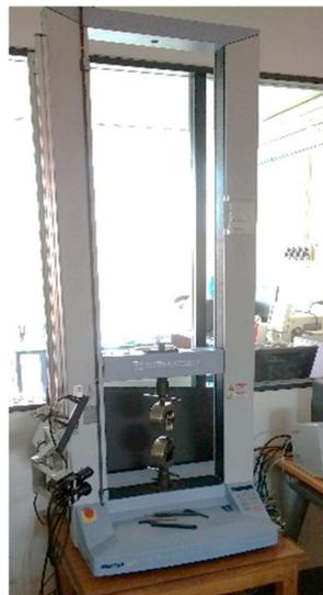
Figure 5. Shimadzu 10 kN tensile testing machine.
