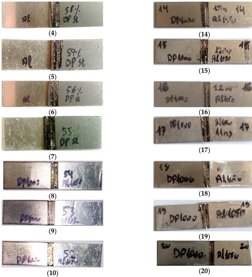
Figure 9. Steel-aluminum welded samples.
