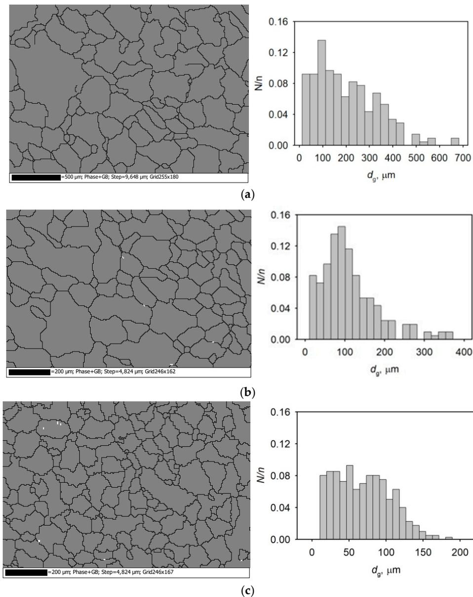
**Figure 2.** EBSD images of the structure and block diagrams of the grain size distribution in the alloy samples: (a) initial state, (b) 0.5 wt.%  $\text{Al}_2\text{O}_3$ , (c) 1 wt.%  $\text{Al}_2\text{O}_3$ .  $d_g$  is the grain size, and  $N/n$  is the ratio between the number of measurements and the number of grains of a certain size.
