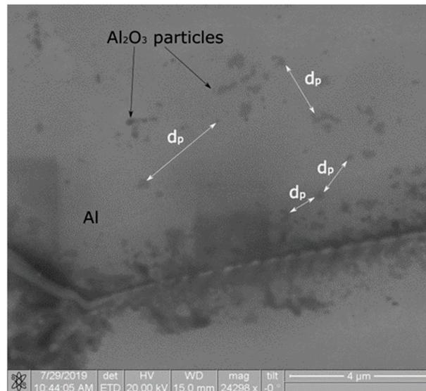
Figure 6. SEM image of the alloy sample with 1 wt.%  $\text{Al}_2\text{O}_3$ .
