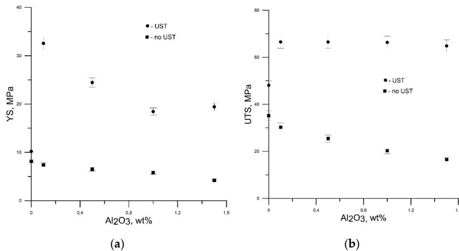
**Figure 5.** The dependencies of (a) the yield stress (YS) and (b) the ultimate tensile stress (UTS) depending on the Al<sub>2</sub>O<sub>3</sub> nanoparticle concentration in the 1100 aluminum alloy.
