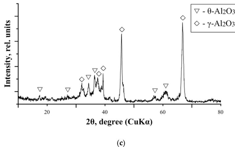
**Figure 1.** TEM image of the structure (a), particle distribution histogram (b), and powder X-ray diffraction [22] (c) of the  $\text{Al}_2\text{O}_3$  nanoparticles.
