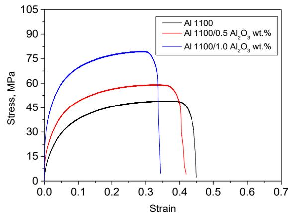
**Figure 4.** Stress–strain curves obtained for the tensile test samples from investigated alloys: Al 1100: Initial state; Al 1100/0.5 wt.% Al<sub>2</sub>O<sub>3</sub>; Al 1100/1 wt.% Al<sub>2</sub>O<sub>3</sub>.
