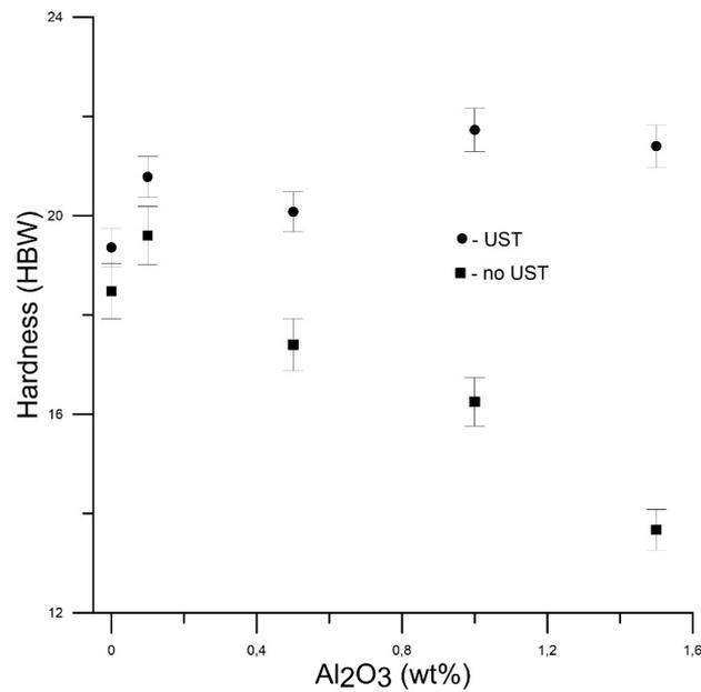
**Figure 3.** The dependence between the Brinell hardness and Al<sub>2</sub>O<sub>3</sub> content in the 1100 aluminum alloy.
