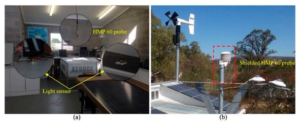
**Figure 3.** (a) Inner space of the office indicating the HMP60 temperature and relative humidity probe and photometer sensor; (b) a setup outdoor weather station indicating the shield HMP60 temperature and relative humidity probe.
