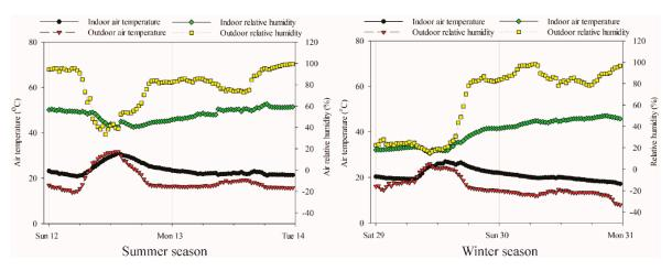
**Figure 9.** Seasonal air temperature and relative humidity response of the passive solar building on a typical clear sky and overcast day.
