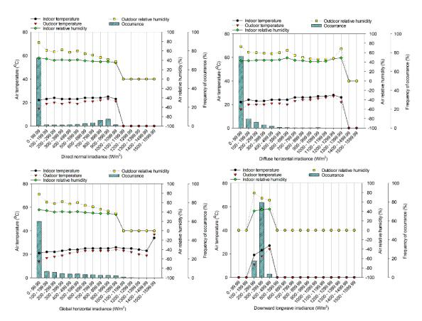
Figure 7. Indoor and outdoor thermal response to various components of solar radiation in summer.
