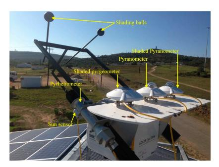
**Figure 2.** SOLY Gear Drive dual-axis sun tracker measuring the selected components of solar radiation in SolarWatt Park, Alice.
