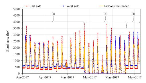
Figure 10. Indoor illuminance distribution of the passive solar building.
