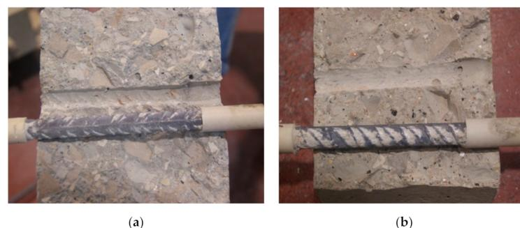
Figure 2. Mobilization of ribs in (a) RC and (b) C100F-Amb.
