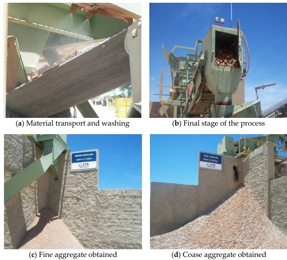
Figure 1. Overview of a RA recycling plant.
