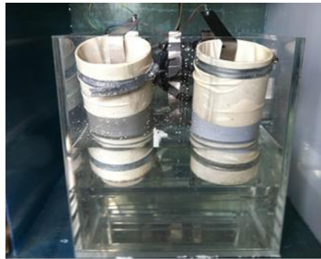
Figure 3. Chloride migration test set up.
