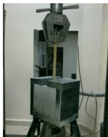
Figure 4. Pull-out test set up.
